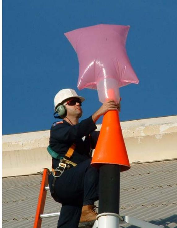
The measurement instruments that are available on the market today are geared towards above ground components, because the leaking component can be totally “encapsulated” by “bagging” the leak and measuring it directly.
