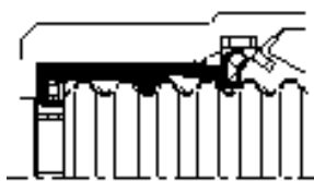
Neo Joint Flexible pipe sealed at bottom of bellows
