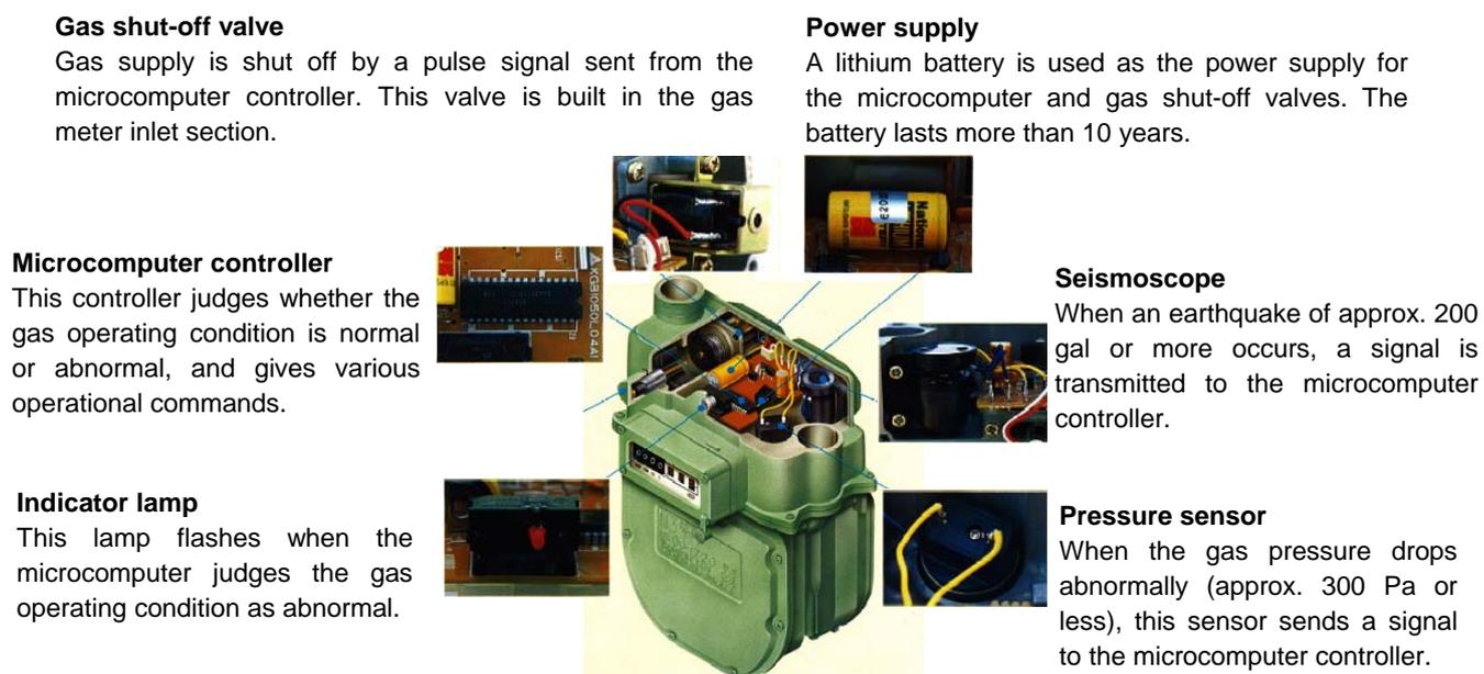
Fig. 1 Construction of intelligent gas meter and function of security components.
