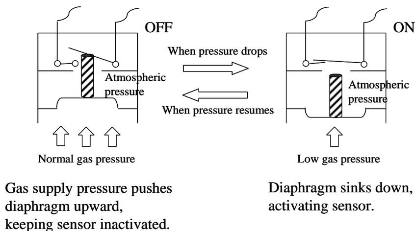
Fig. 2 Construction and operating principle of pressure sensor.
