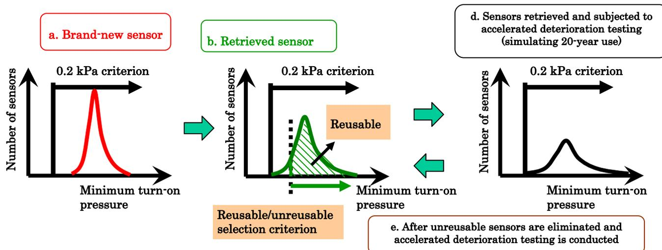
Fig. 3 Basic procedure for pressure sensor characteristic evaluation.
