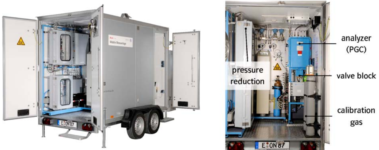
Fig. 4: Mobile measurement vehicle of Open Grid Europe with GC9000 PGC of RMG admissible for use in verification measurements.
