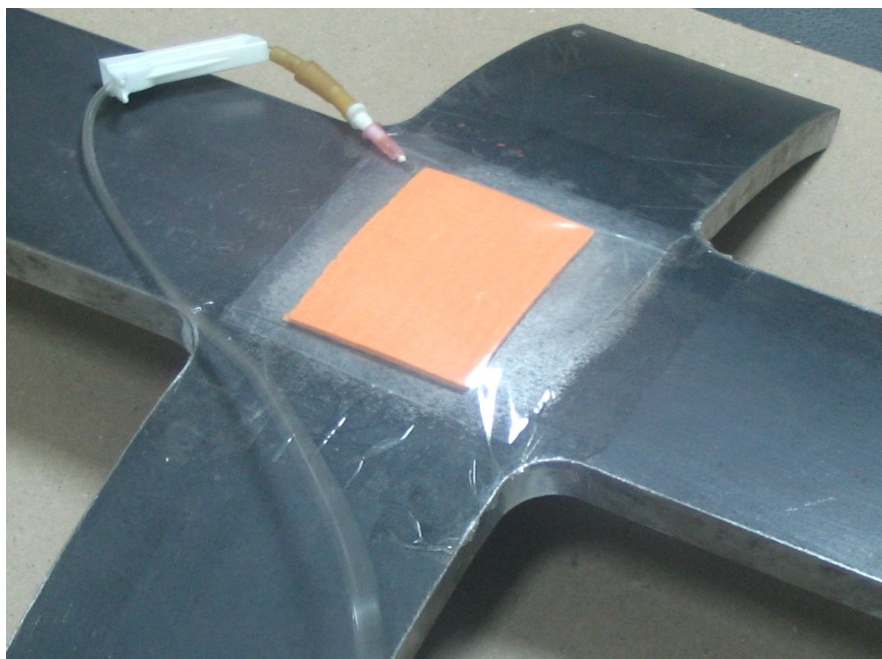
Figure 1 – SCC test sample with corrosion unit to simulate separation of insulation cover on pipes
