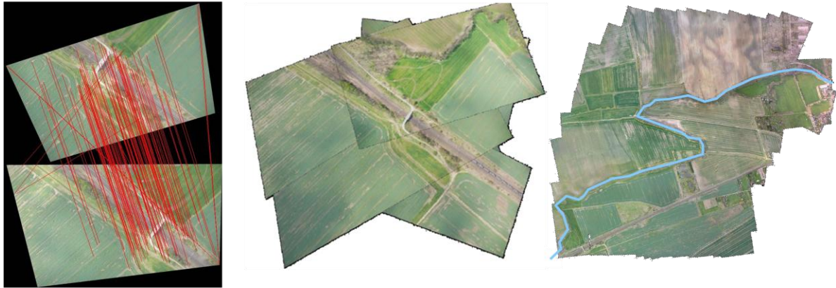
Figure 6: Example of image georeferencing and assembling
