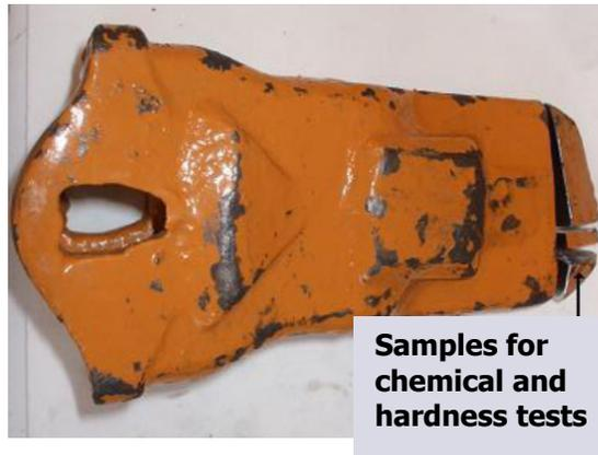
Figure 3.2.2: **Samples taken from a tooth for chemical and hardness analysis**
