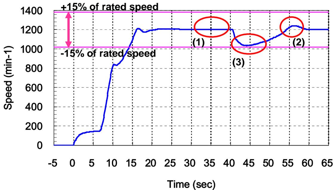
Figure 6 The engine speed behavior of the first step loading from starting
