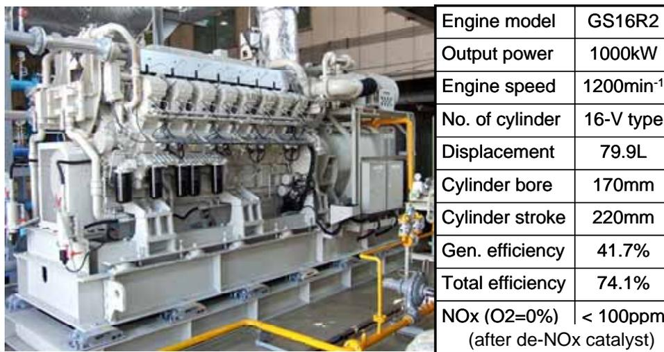
Figure 2 The appearance and specifications of GS16R2 gas engine
