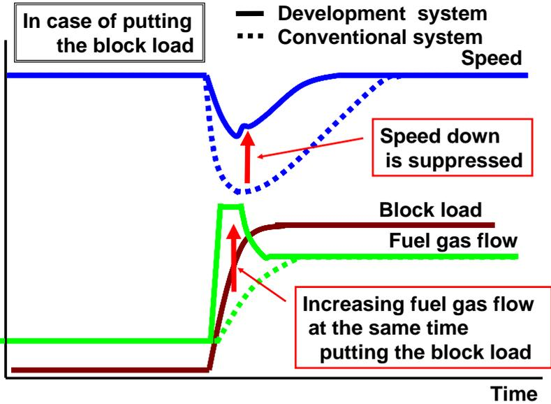
Figure 5 The compensation control during loading of the integrated controller
