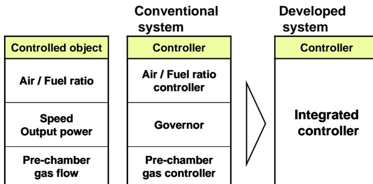
Figure 4 The development of the integrated controller
