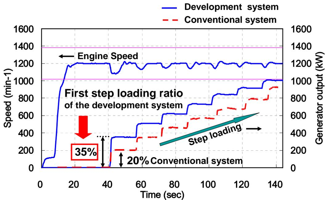
Figure 10 Step loading results in case of a power failure
