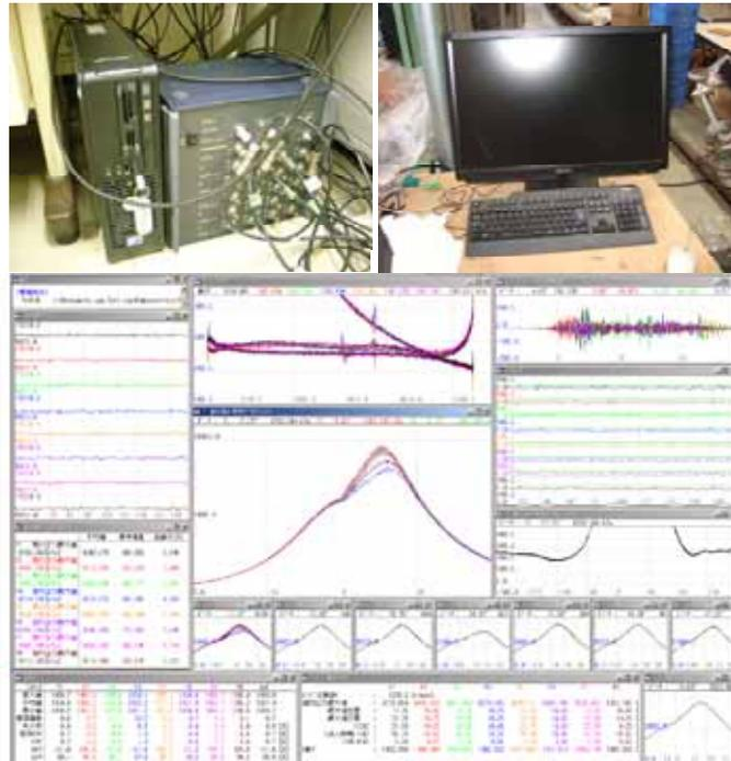
Figure 7 The combustion analyzing system
