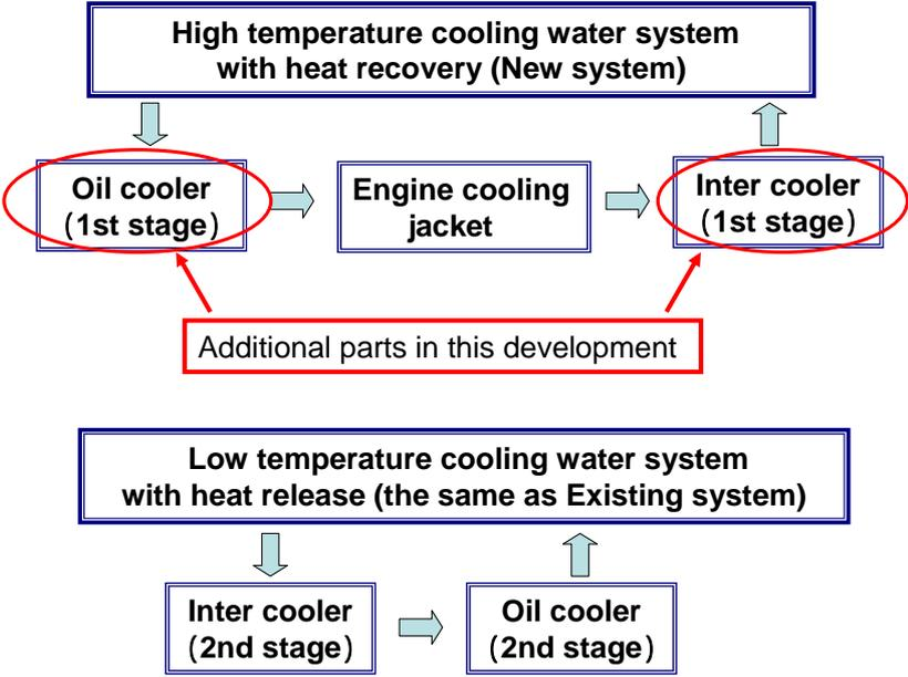
Figure 11 The development of new heat recovery system
