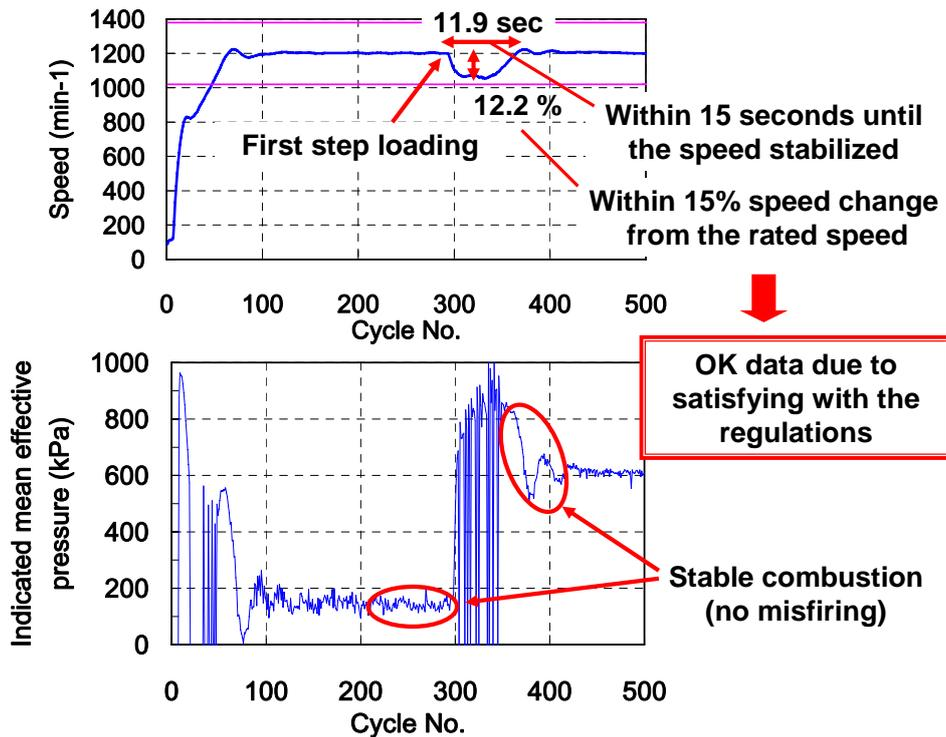
Figure 9 OK data of the first step loading (after adjusting engine parameters)
