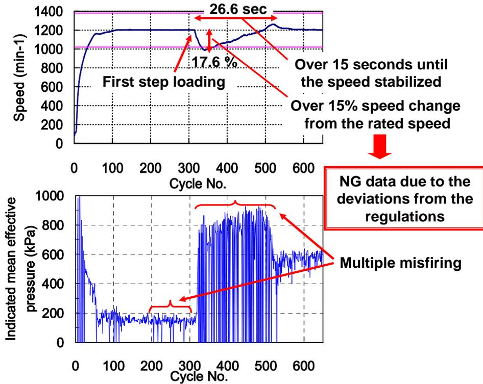
Figure 8 NG data of the first step loading (before adjusting engine parameters)
