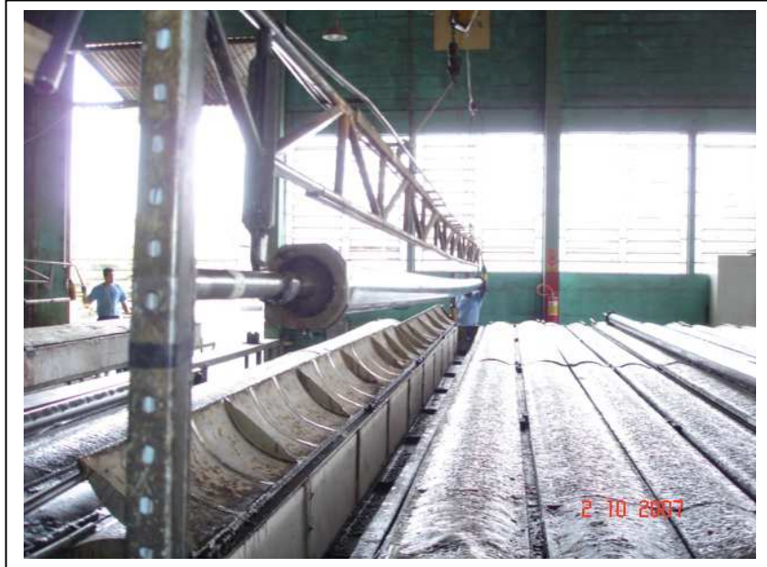
Figure 1: Electric hothouses of cure and post-cure – material's loading
