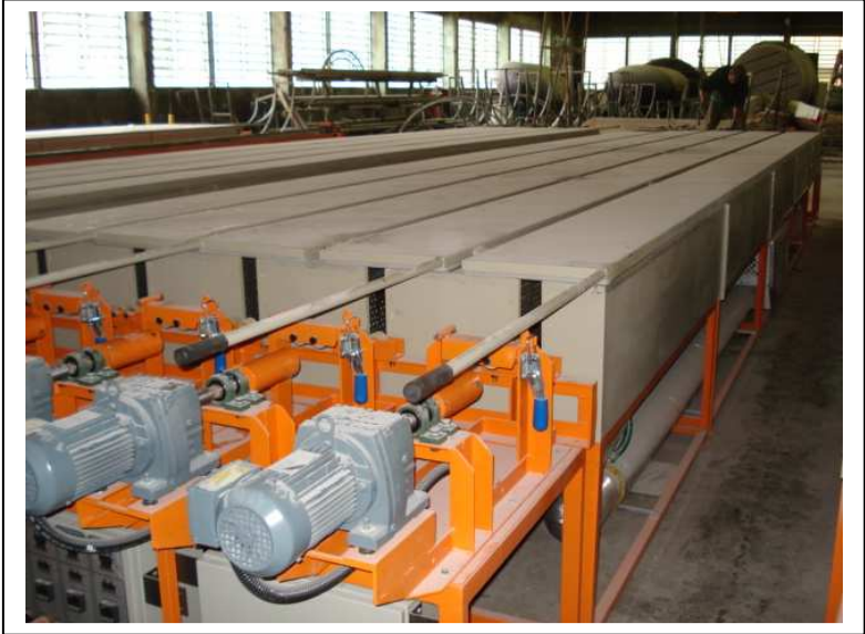
Figure 4: Hothouses of cure and post-cure by natural gas developed – in operation
