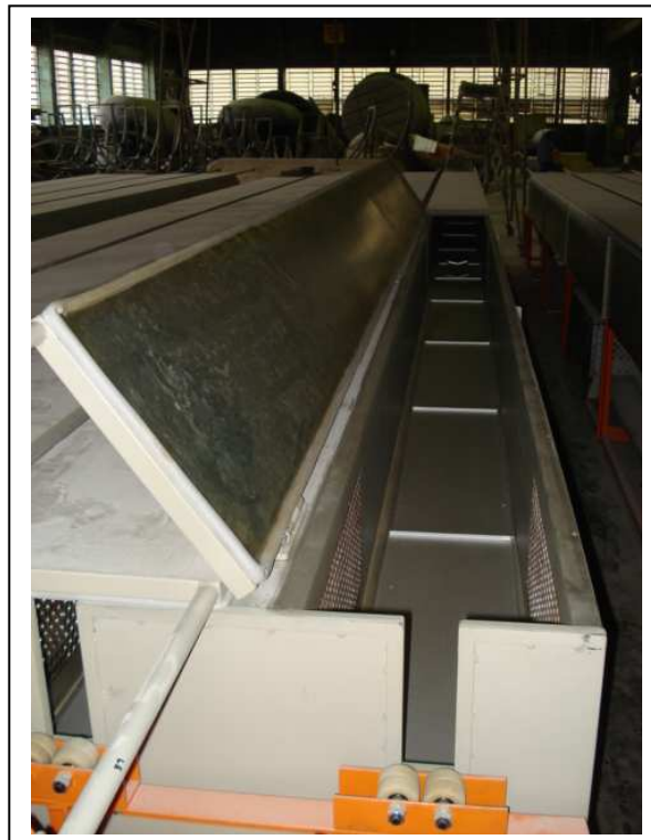
Figure 3: Hothouses of cure and post-cure by natural gas developed – without load
