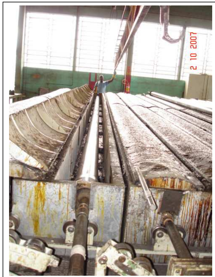
Figure 2: Electric hothouses of cure and post-cure – mandrel placed
