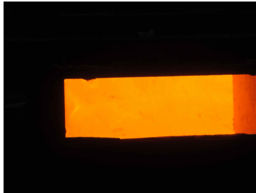
FIG. 4 Flameless combustion of the self-regenerative burner in the test furnace ( O_2=3\% )
