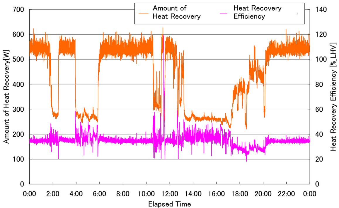
Figure 8. Heat recovery characteristics during one-day operation at a resident.
