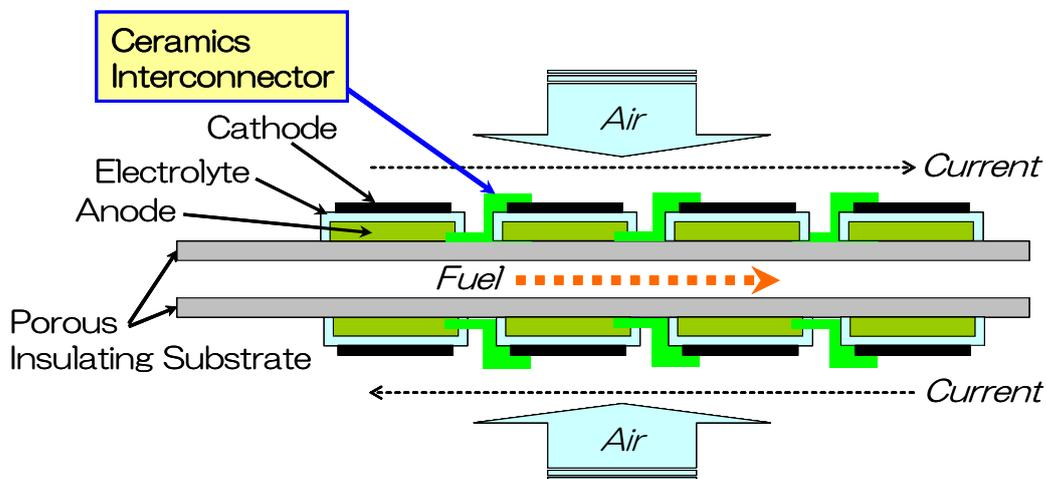
Figure 1. Sectional diagram of all-ceramics-segmented cell stack.
