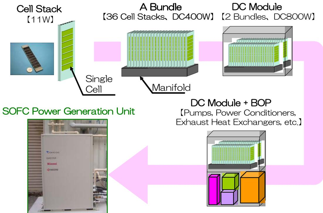
Figure 2. Procedure of assembling SOFC power generation unit.
