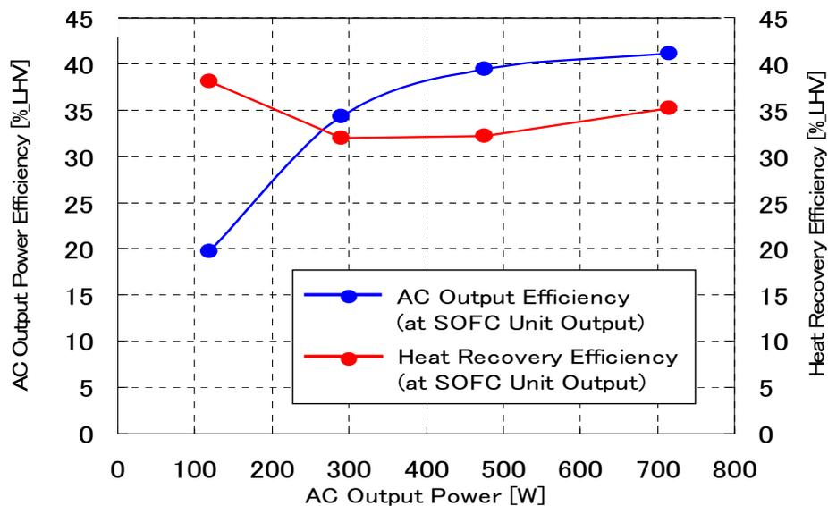
Figure 4. Basic performance of SOFC power generation unit.
