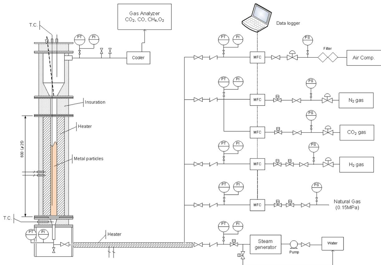
Fig. 3 Schematic diagram of CLC test system
