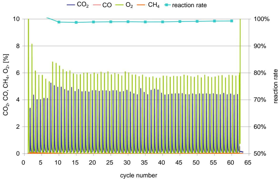
Fig. 7 Gas analysis of continuous redox test (case3-1)
