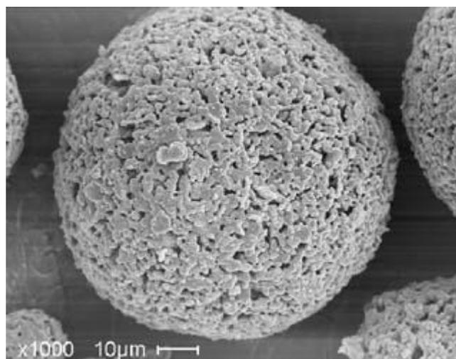
Fig. 4 Metal particles (oxygen carrier)
