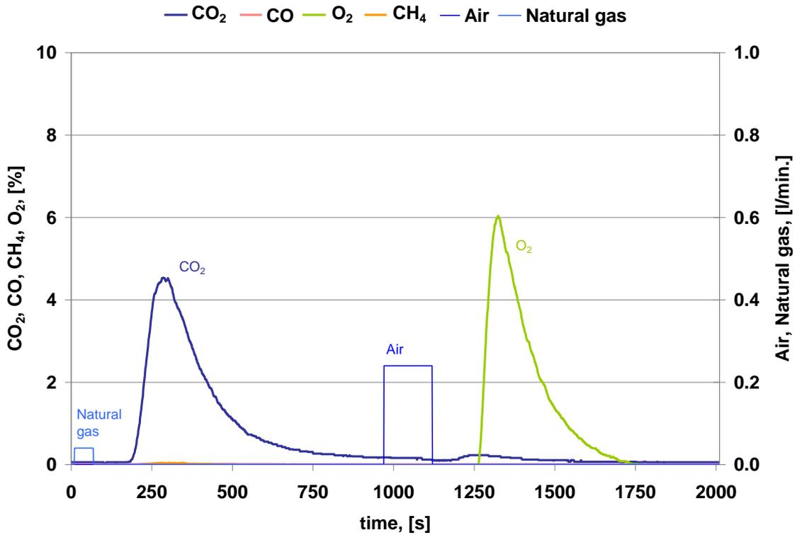
Fig. 6 Gas analysis of redox test (case3-1)
