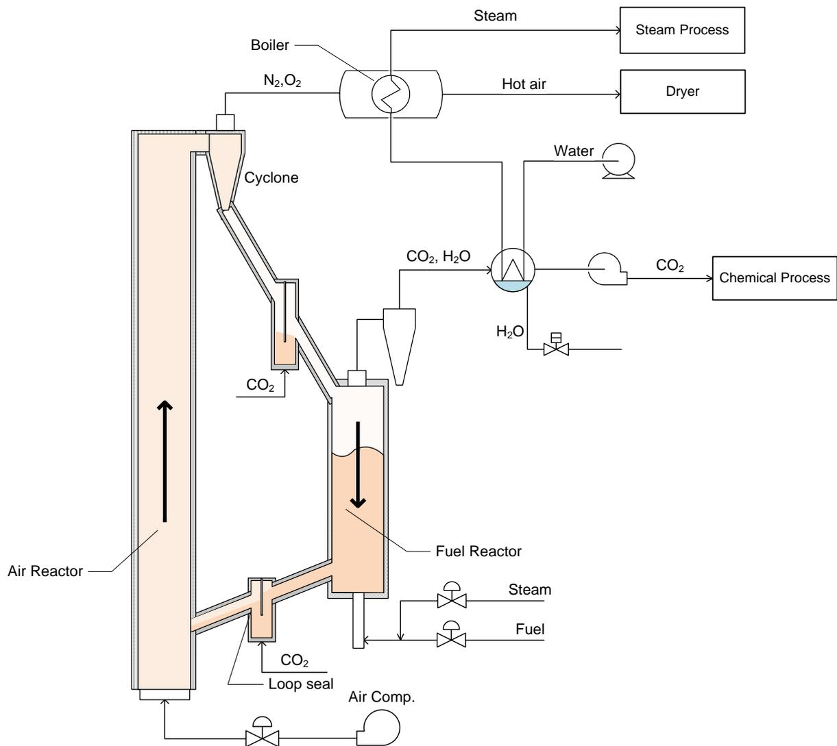
Fig. 8 CLC boiler system
