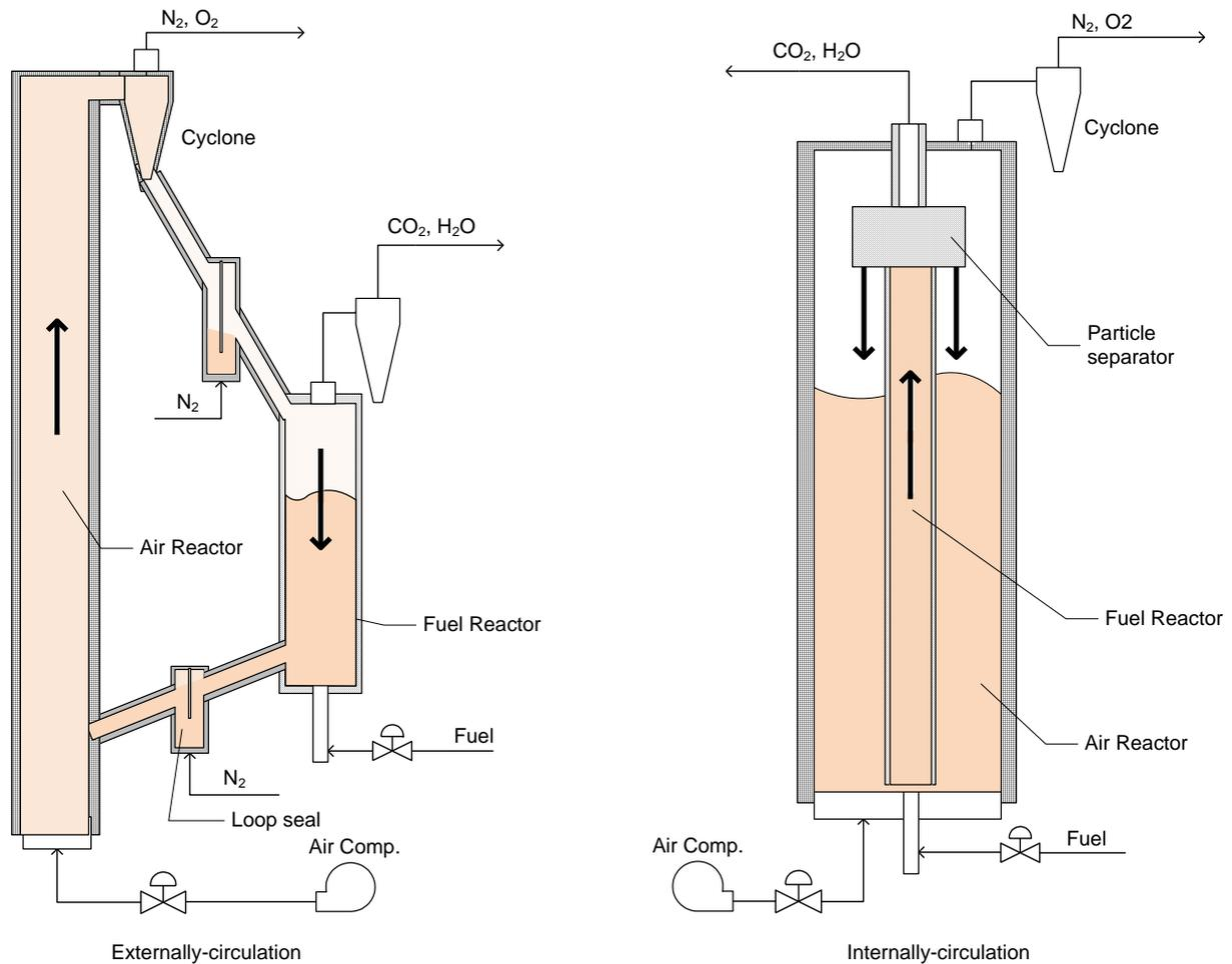
Fig. 2 Comparison of cycle system
