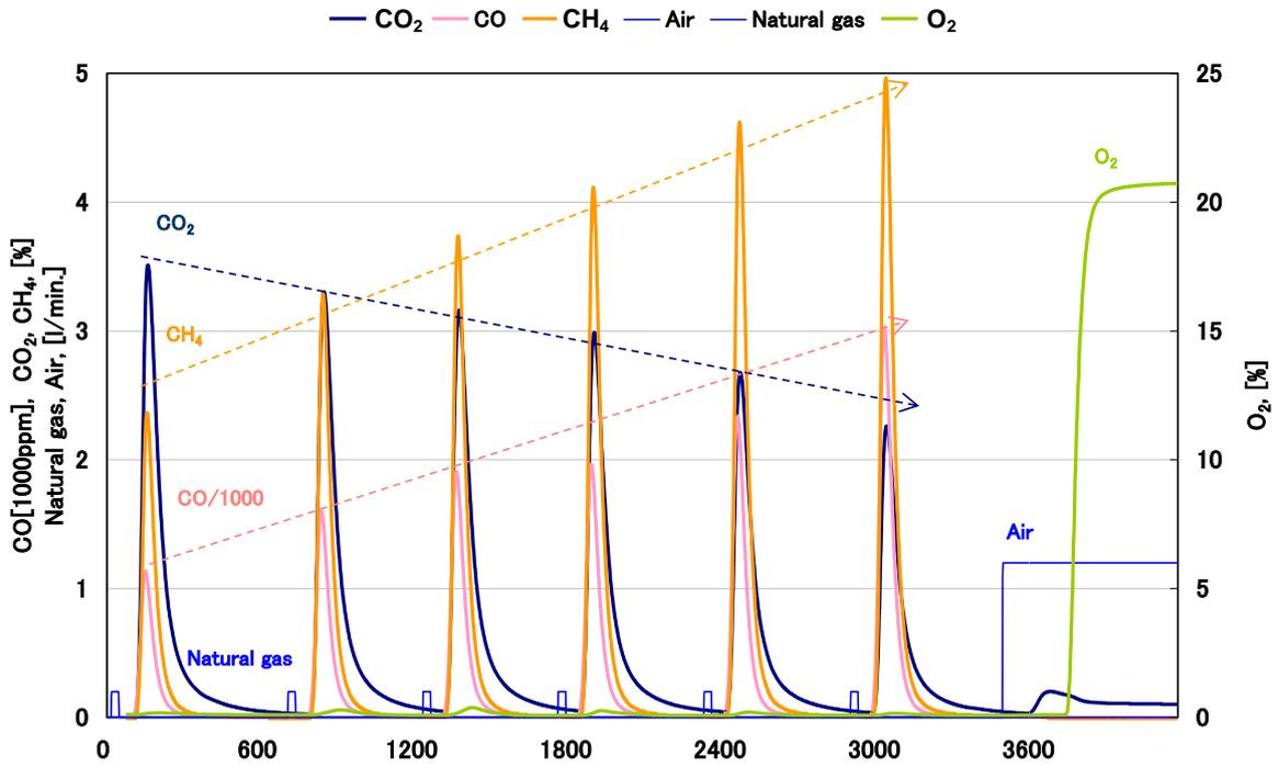
Fig. 5 Gas analysis of continuous reduction test (case1-2)
