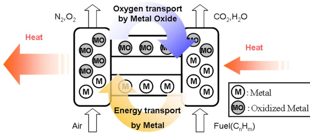
Fig. 1 Conceptual diagram of Chemical Looping Combustion
