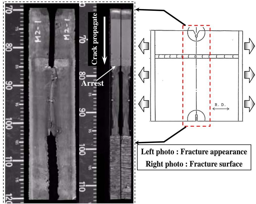
Fig. 6 Example of fracture surface of duplex ESSO test (25mmt, -196deg.C)
