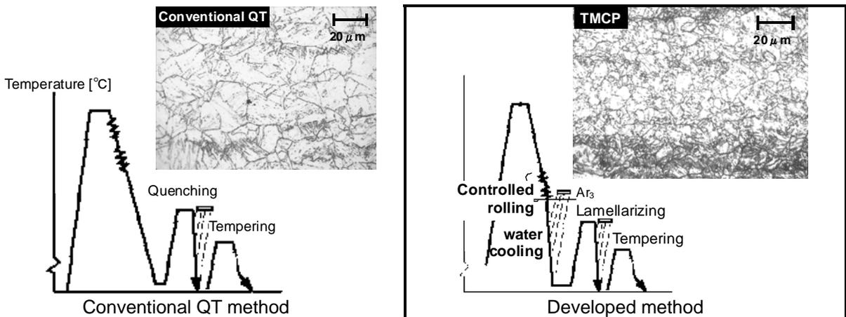
Fig. 3 Generals of production process and typical microstructure
