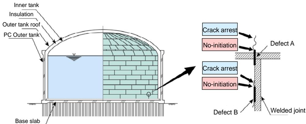
Fig. 1 Requisite properties for material of LNG tank<sup>11</sup>
