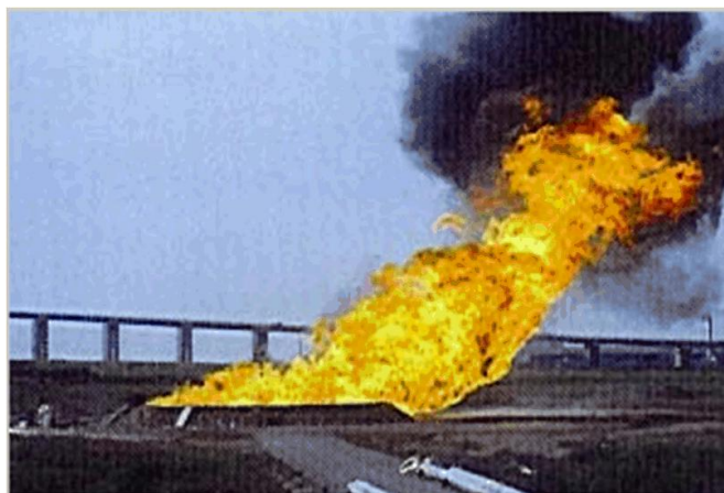
Figure 12: The experiments of Montoir highlight the influence of soot formation for large pool fire.
