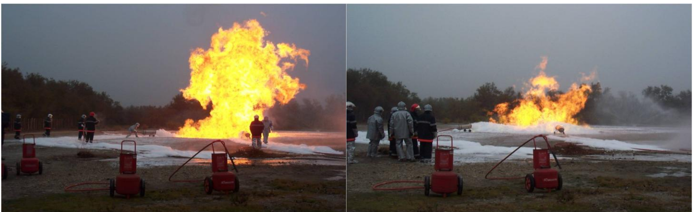
Figure 10 : These two pictures illustrate the efficiency of foam addition on flame size.
