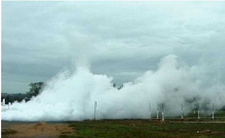
Figure 6: LNG vapor cloud from a pool – the vapor cloud is first very closed from the ground due to its density and then rise due to buoyancy and passive dispersion
