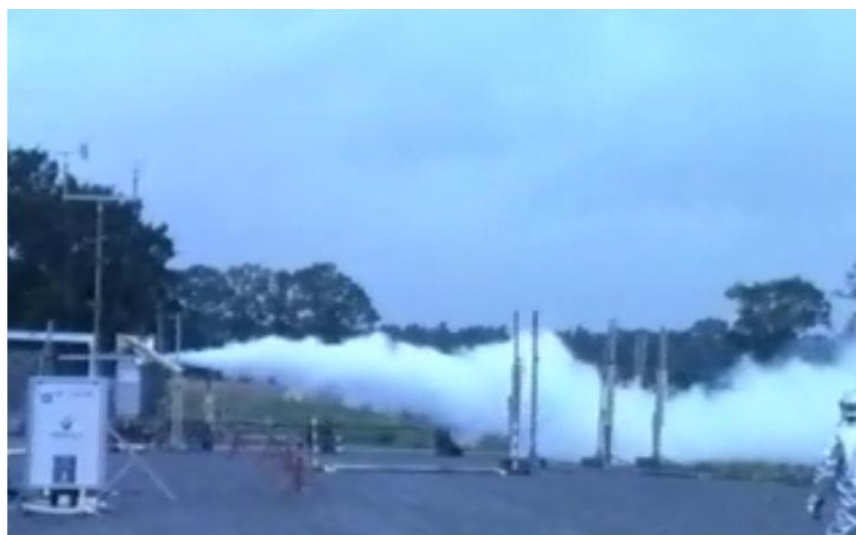
Figure 7: LNG pressurized jet – the jet is first horizontal above ground due its initial velocity, then fall to the ground due to gravity and finally rise due to buoyancy and passive dispersion
