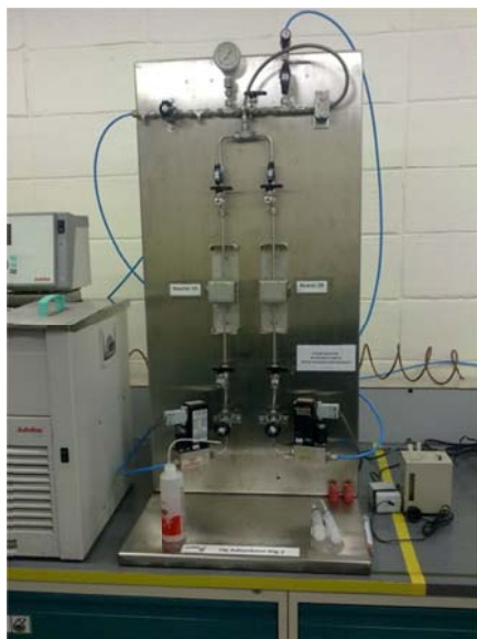
Figure 5: A typical screening reactor for SSIL evaluation in PETRONAS.
