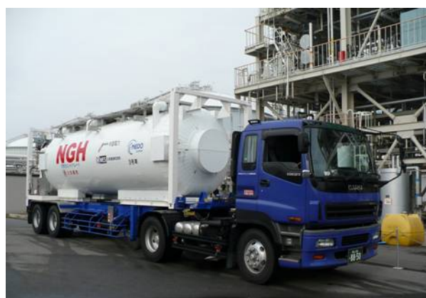
Figure 12: 7.5 capacity purpose-built tank truck equipped with re-gasification device
