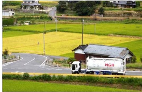
Figure 16: NGH purpose-built tank truck delivering NGH to non-pipeline area
