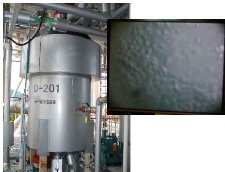
Figure 9: NGH reactor and slurry generated inside
