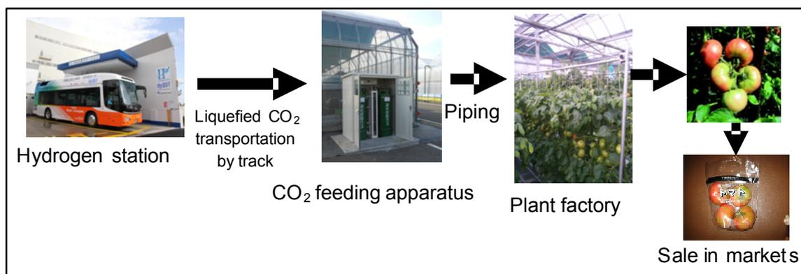
Figure 6. Schematic flow of CO<sub>2</sub> utilization for tomato plant factory.
