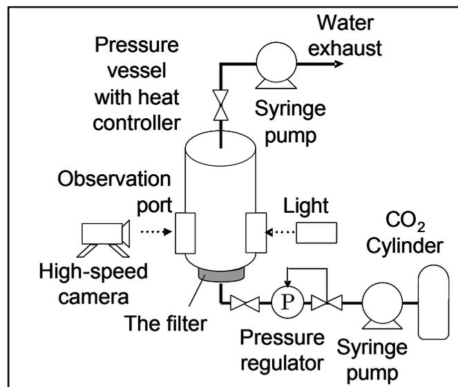
Figure 8. Schematic of experimental apparatus.
