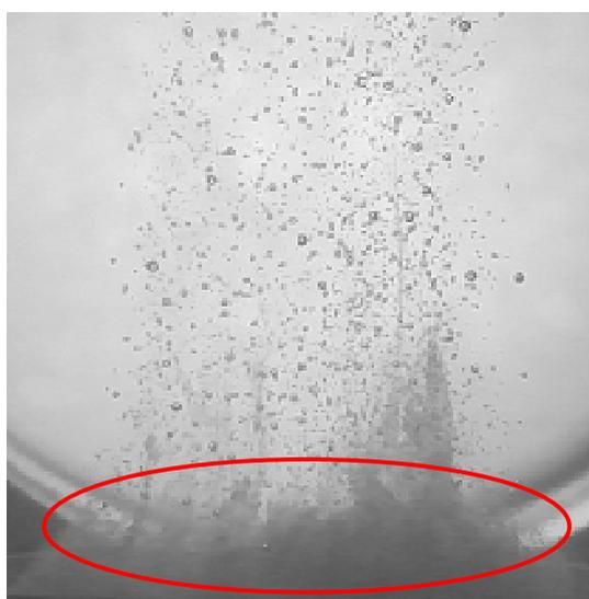
Figure 9. Behavior of injected CO<sub>2</sub> microbubbles (40 °C, 10 MPa).
