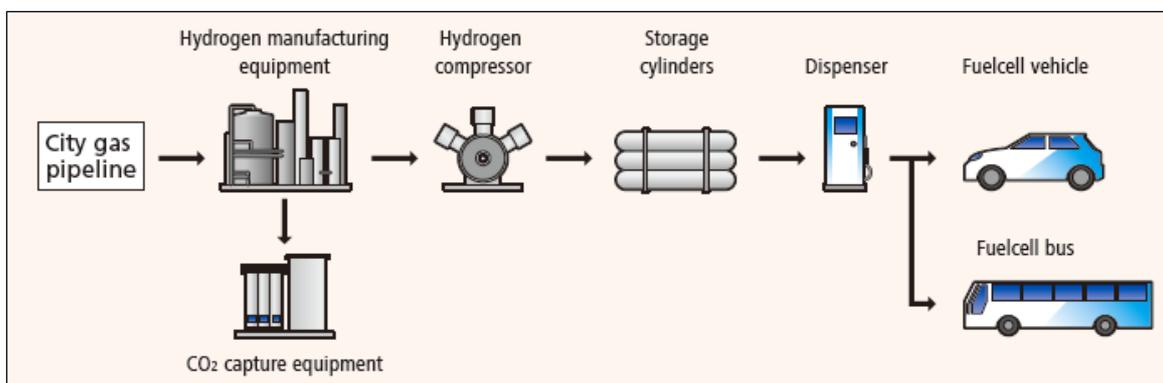
Figure 5. System flowchart of the hydrogen station with CO<sub>2</sub> capture equipment.
