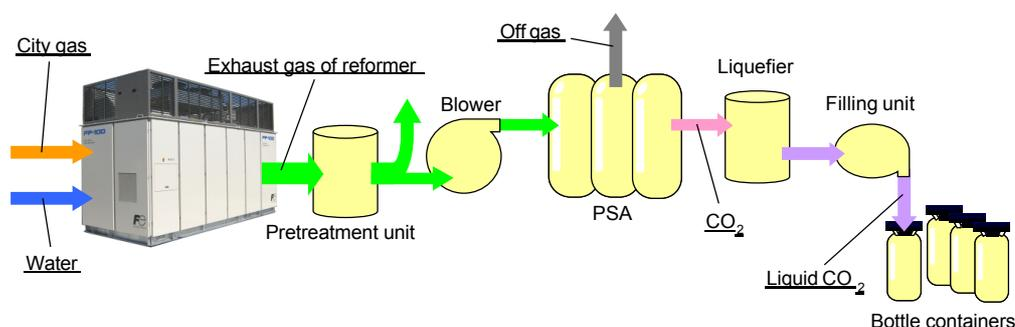
Figure 3. System flowchart of the CO<sub>2</sub> recovery equipment in the PAFC system.
