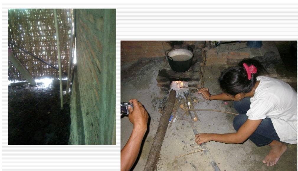
Figure 4. Biogenic gas is directly used for cooking using iron tube at its end. The example is from a rural household in Sragen, also Central Java (Foto courtesy of Gas Working Group)
