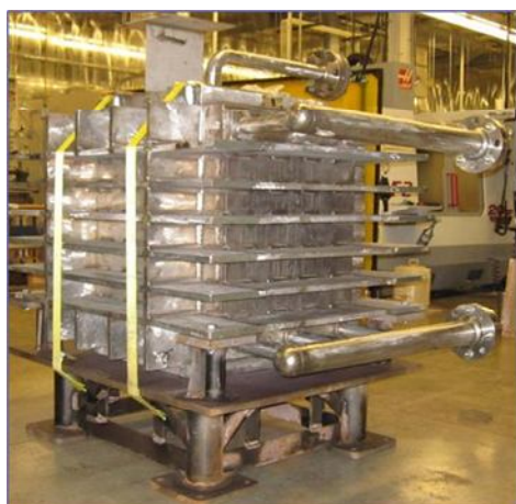
Figure 6. Fabricated 25 bpd microchannel FT reactor and 130 bpd concept
