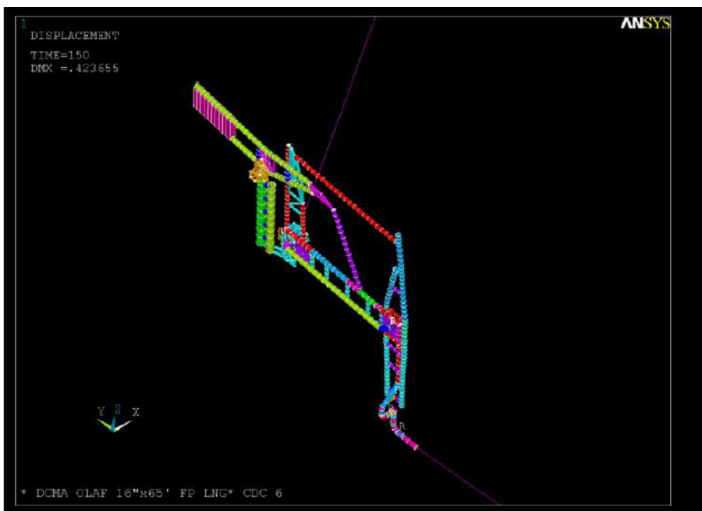
Figure 14: OLAF time domain dynamic calculation on ANSYS FEA software
