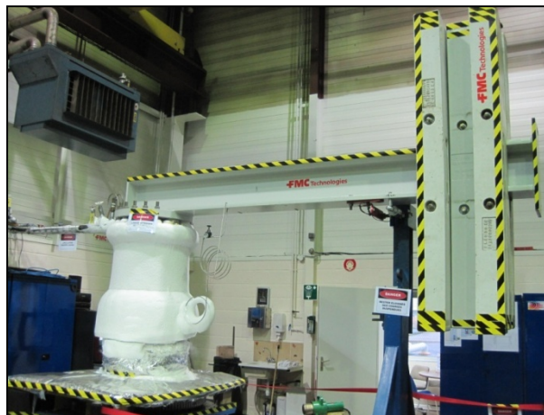
Figure 6: The Chiksan 24” Constant Motion LNG Swivel Joint during running test with external load applied
