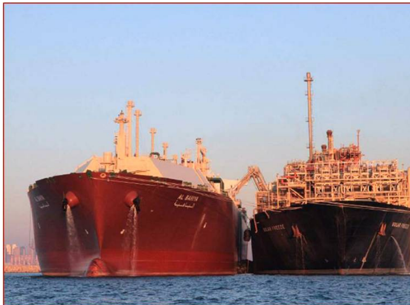
Figure 3: Side-by-side LNG transfer with Chiksan Loading Arms in Dubai
