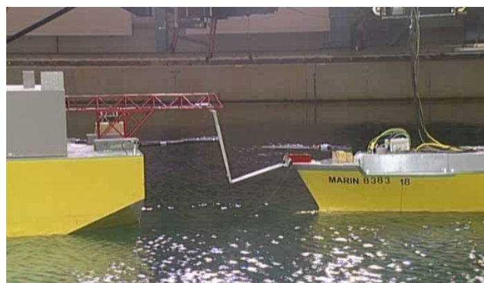
Figure 17: offloading basin tests – Tandem
