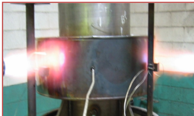
Figure 7. The Chiksan Swivel Joint during fire safe qualification testing
