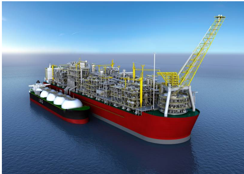
Figure 1 Shell's Prelude FLNG concept
