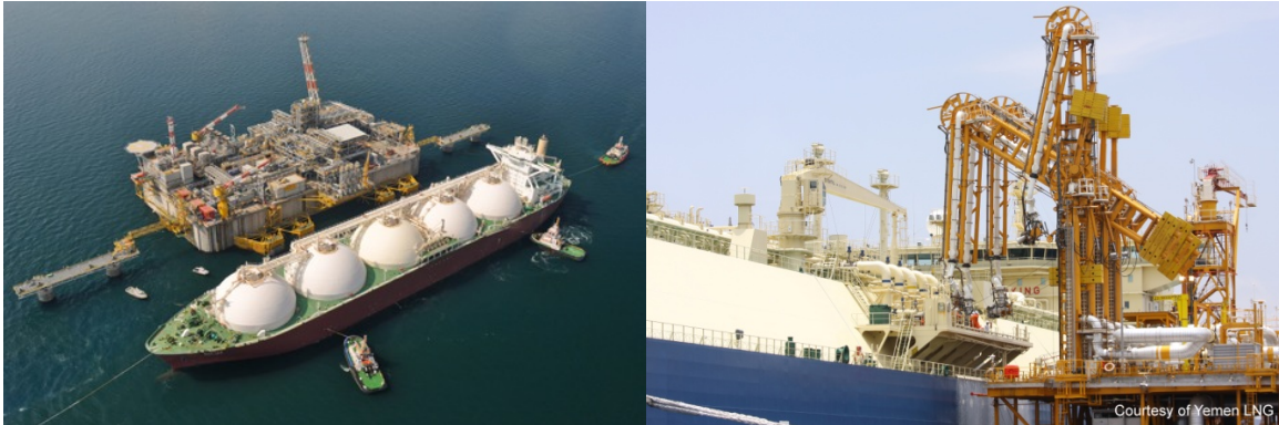
Figure 3 and 4: Chiksan LNG arms with Targeting System on GBS and exposed location applications
