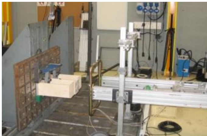
Figure 10: Small dynamic setting for simplified boxes (13 kg impactor at approximately 8 m/s)
