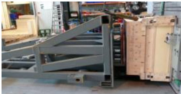
Figure 12: Crash-test for full box system (2T impactor at 4 m/s)
