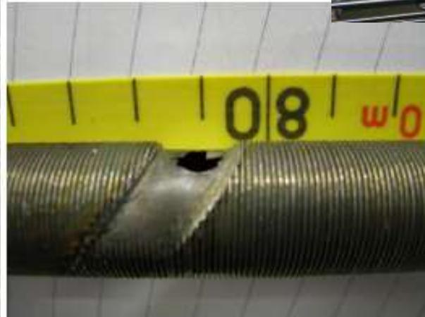
Failure mode was wear of the tubes against baffle plates caused by flow induced vibration
