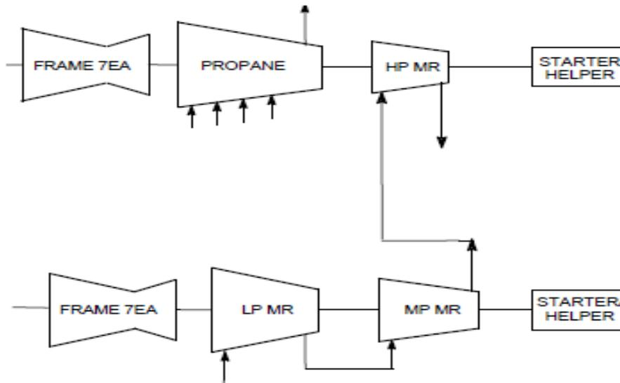
Figure 1. Two Frame 7EA Gas Turbines Used for C<sub>3</sub>MR/SplitMR™ Cycle [1]
