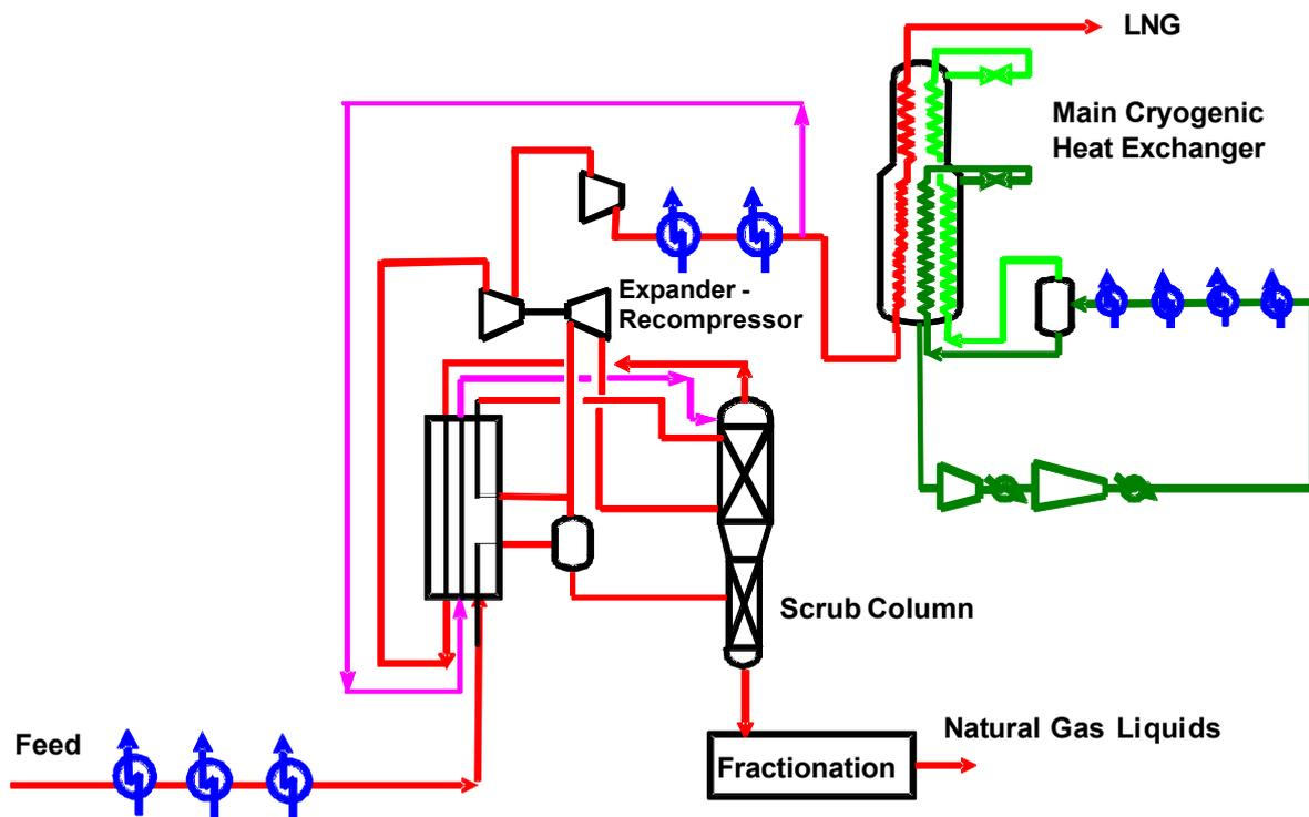
Figure 3. Expander-Recompressor LPG Recovery Process for  $C_3MR$  LNG Process [7]
