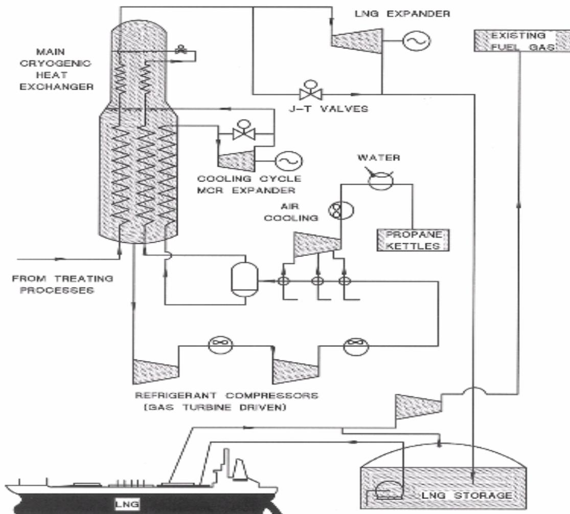
Figure 2. Liquid Expanders for C<sub>3</sub>MR Cycle LNG Plant [6]
