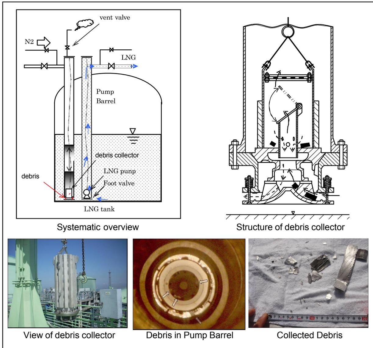
Figure 4.5 Pump Barrel Debris Collection Jig and Collected Debris
