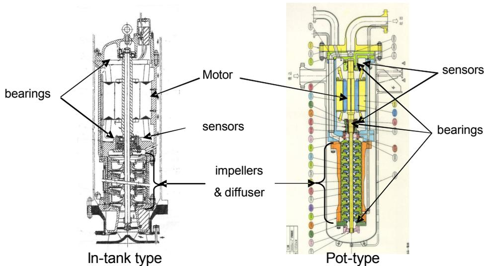
Figure 2.1 LNG Pump Structure Schematic Diagram
