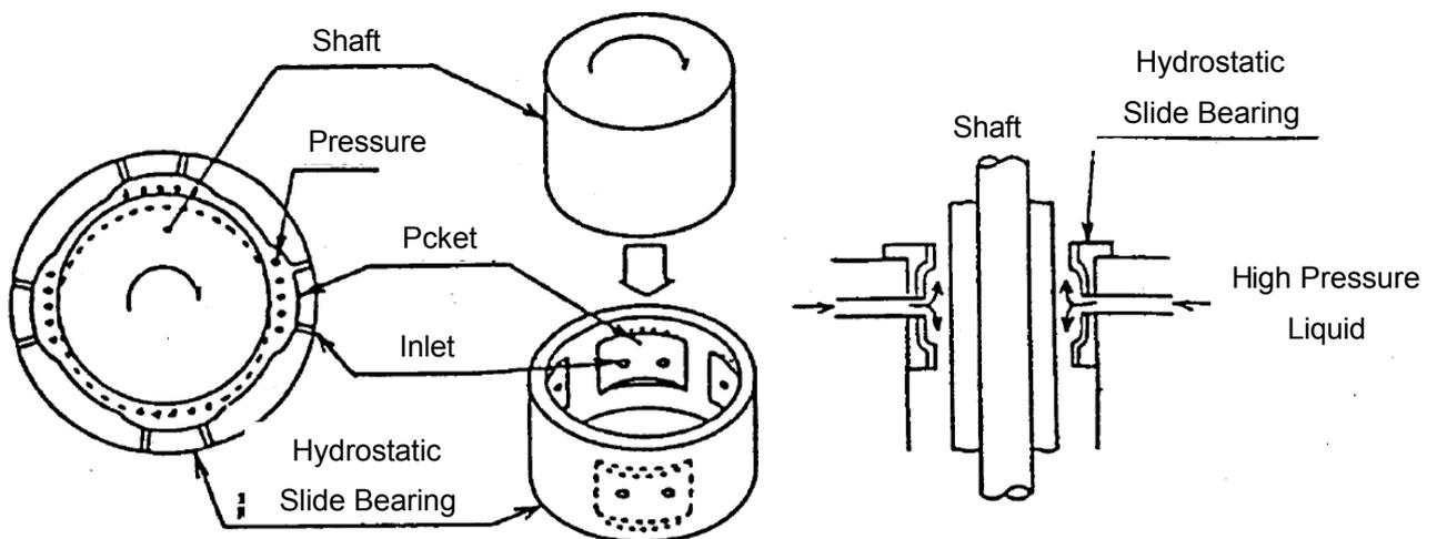
Figure 5.1 Hydrostatic Slide Bearings Schematic Diagram
