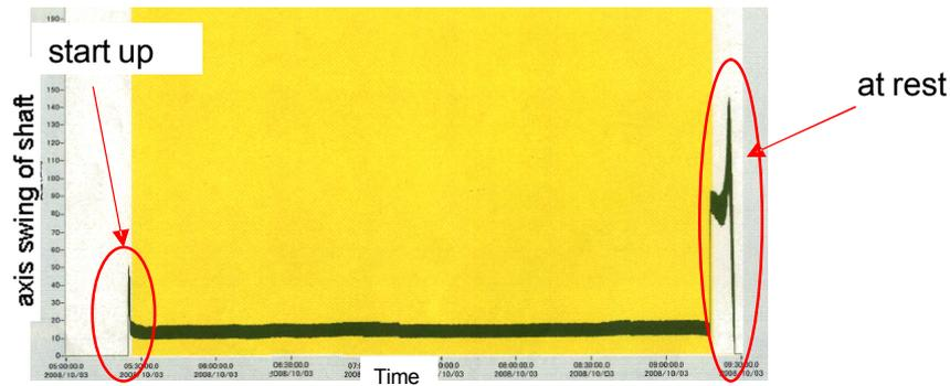
Figure 5.2 Hydrostatic slide Bearing Type Pump Axis Displacement Sample Monitoring Data
