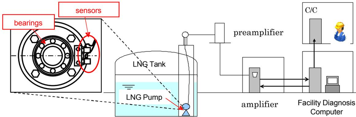
Figure 3.1 Vibration Monitoring System Schematic Diagram
