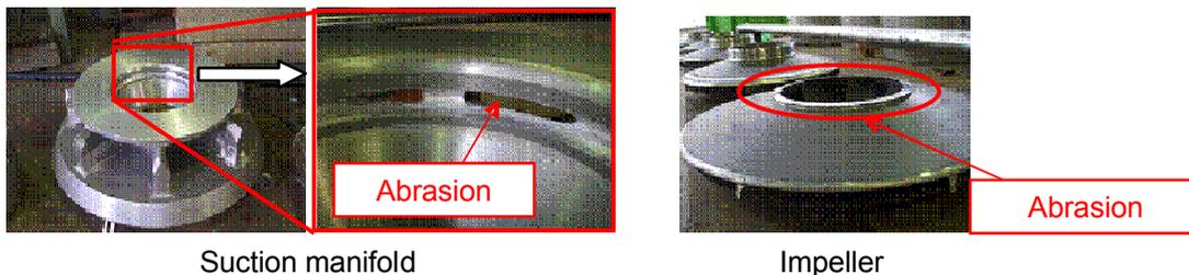
Figure 4.1 In-tank Pump Damage Example -1
