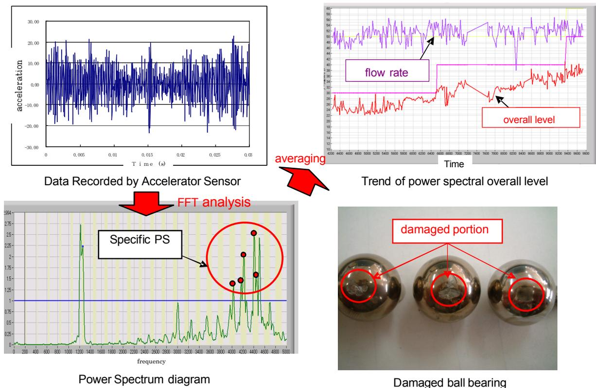
Figure 3.2 Sample Acceleration Data
