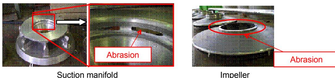
Figure 4.1 In-tank Pump Damage Example -1
