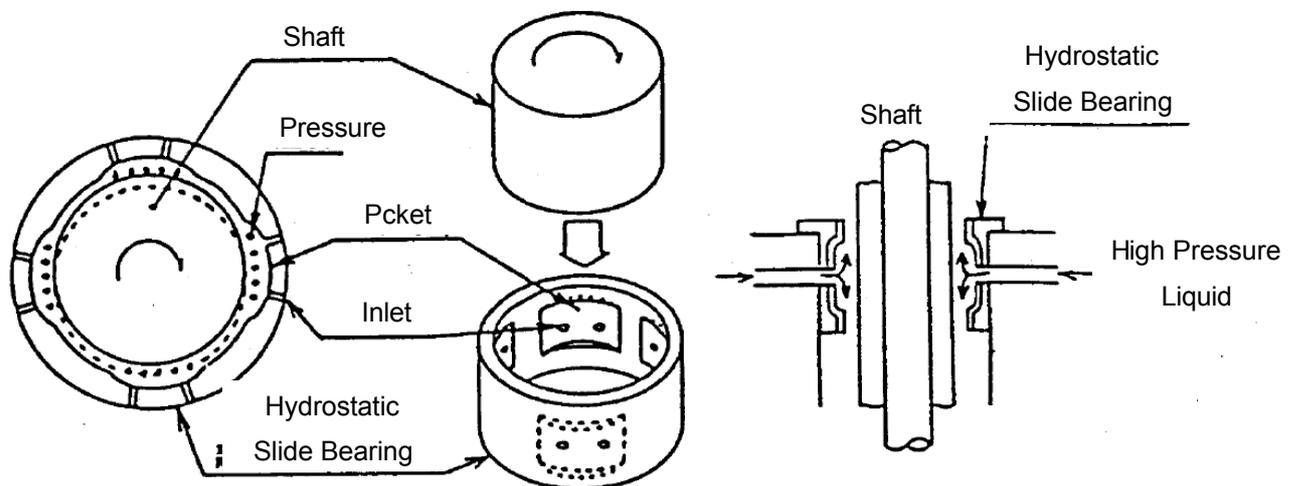
Figure 5.1 Hydrostatic Slide Bearings Schematic Diagram
