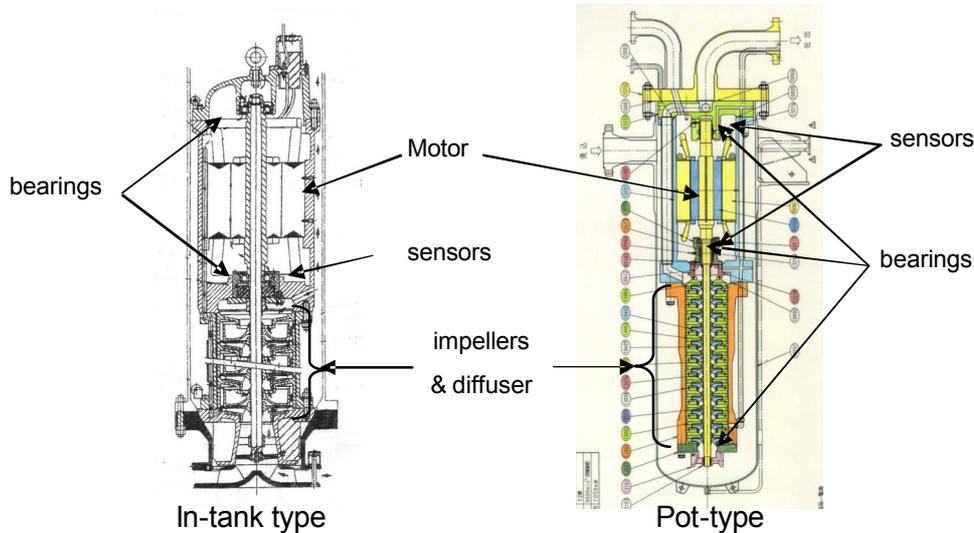
Figure 2.1 LNG Pump Structure Schematic Diagram
