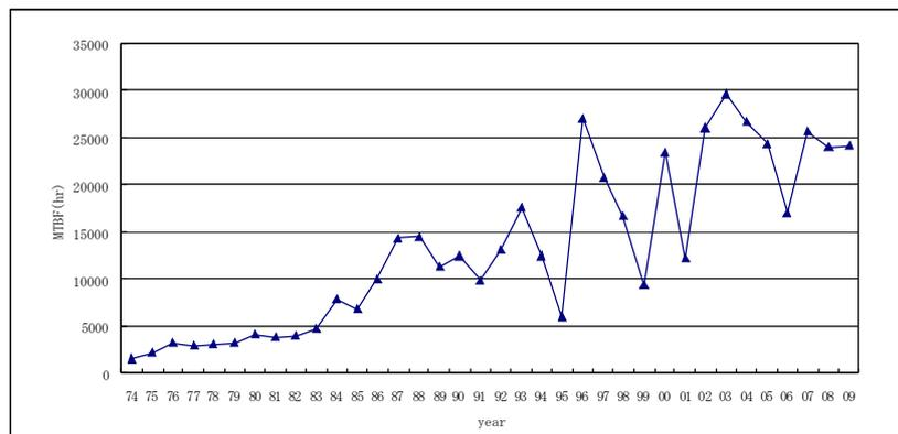
Figure 2.2 MTBF at the Sodegaura LNG Terminal (1974-2009)
