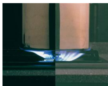
Figure 5.33 Comparison of high efficiency [L] and conventional [R] burners
