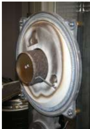
Low NOx Burner
