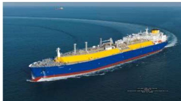
Large Diesel driven LNG carrier with dual fuel capability.
