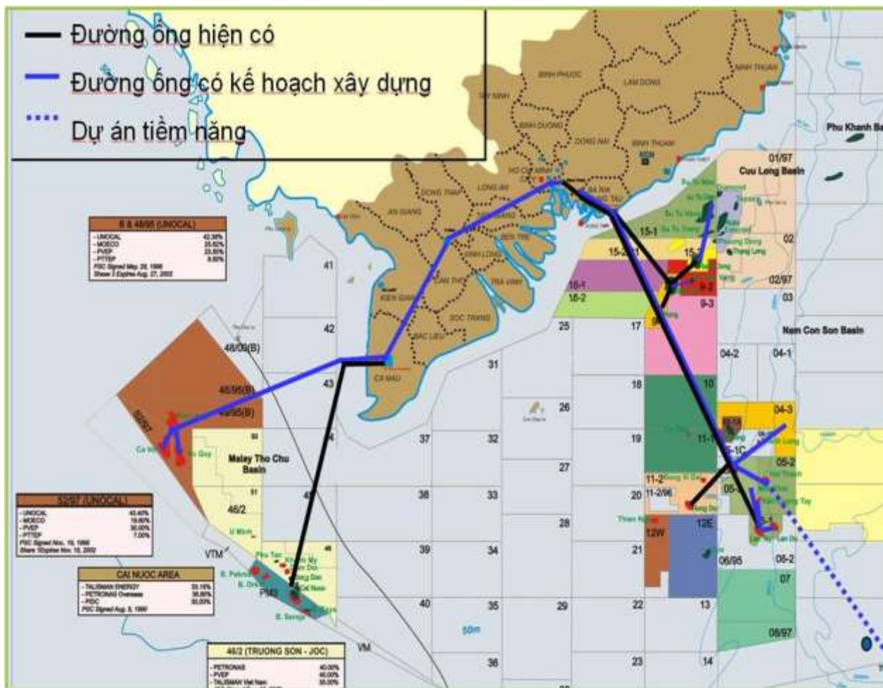
Gas pipeline system in Vietnam (Source: Hien, 2010) (black = existing, blue = under development, dotted blue = potential)
