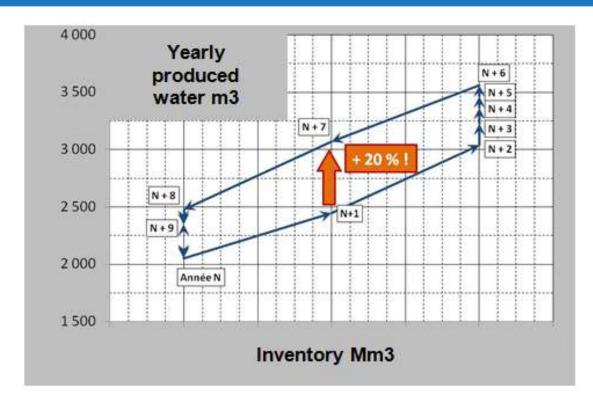
Quasi reversible mode when working gas (WG) produced is « small »
