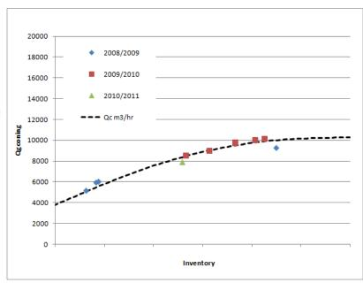
For each well, analysis of the 3 last campaigns to determine « observed » critical rate as a function of inventory
