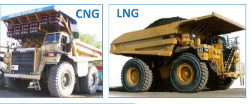
**Coal Mines** Super HD mine hauling trucks (dual fuel or dedicated, CNG or LNG) were successfully tested during past two decades in the USA, Ukraine and Russia.
