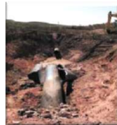
(Algeria), pipeline Hassi-R'mel-Arzew Mohammadia, corrosion - flight of gas explosion-fire, 78 persons hurt, damage to property - similar to a previous accident le 19 in August, 2004
