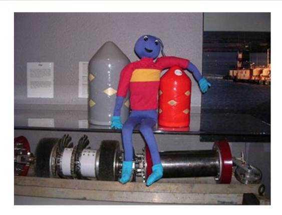
A "pig" is a scraping tool that is sent through a pipeline to clean it out. "Smart pigs" have sensors that can detect cracks or corrosion in the pipeline, helping to prevent leaks.
