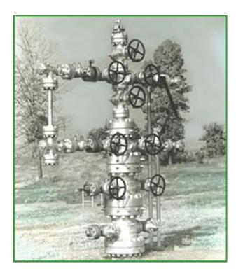
A Christmas tree is a set of valves, pipes, and fittings used to control the flow of oil and gas as it leaves a well and enters a pipeline
