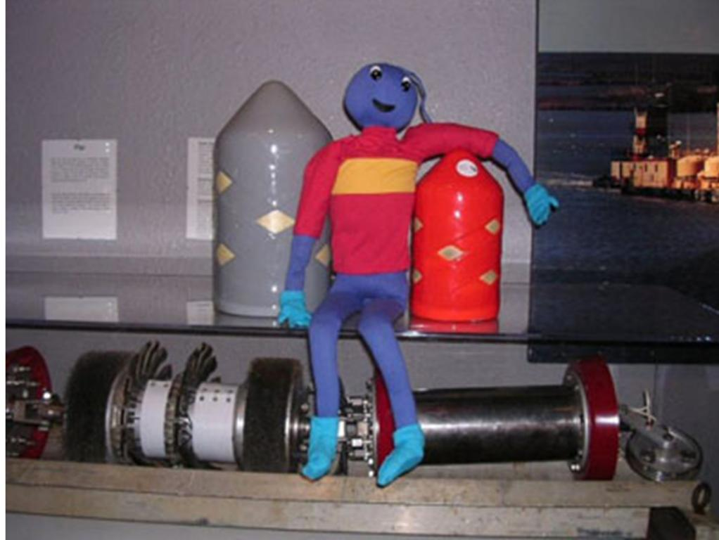
A "pig" is a scraping tool that is sent through a pipeline to clean it out. "Smart pigs" have sensors that can detect cracks or corrosion in the pipeline, helping to prevent leaks.
