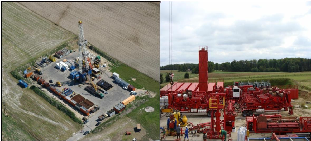
Fig. 5. Lubocino-1 well drilling pad (left); fracking job at Lubocino-1 well (right)
