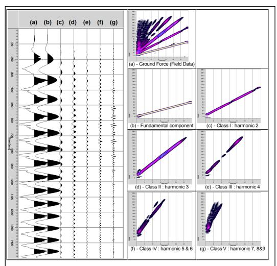
Figure 7: Example of Ground force decomposition in 5 classes using Adaptive filter method. Left: Time representation of 1.5s of the GF as input with its components as results. Right: F-T projection of each corresponding signal.
