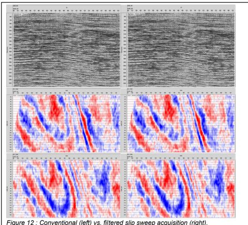
Figure 12 : Conventional (left) vs. filtered slip sweep acquisition (right).
