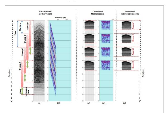
Figure 2: Slip sweep method. (a) uncorrelated mother gather composed of four sweeps, (b) F-T projection of one trace from (a), (c) correlation of (a), (d) F-T projection of one trace from (c), (e) split correlated individual records.
