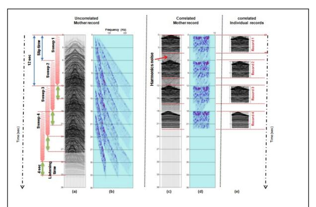
Figure 4: Slip sweep and harmonics problem. (a) uncorrelated mother gather composed of four sweeps, (b) F-T projection of one uncorrelated trace from (a), (c) correlation of (a), (d) F-T projection of the same trace in (b) after correlation, (e) split correlated individual records.
