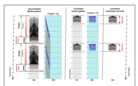
Figure 1: Conventional method. (a) uncorrelated mother gather composed of two sweeps, (b) F-T projection of one trace from (a), (c) correlation of (a), (d) F-T projection of one trace from (c), (e) split correlated individual records
