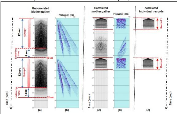
Figure 3: Conventional method. (a) uncorrelated mother gather composed of two distorted sweeps, (b) F-T projection of one distorted trace from (a), (c) correlation of (a), (d) F-T projection of the same trace in (b) after correlation, (e) split correlated individual records.
