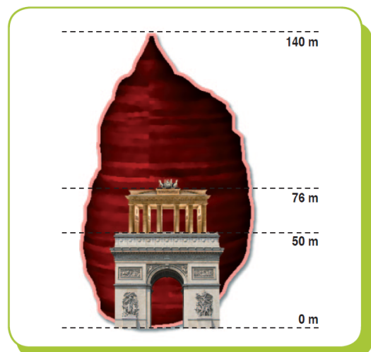
Fig. 3: Typical salt cavern for natural gas storage
