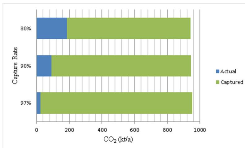
Figure 4. CO<sub>2</sub> emissions with different capture rates [10].
