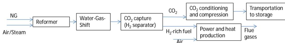
Figure 2. Block diagram for pre-combustion CO<sub>2</sub> capture [10].
