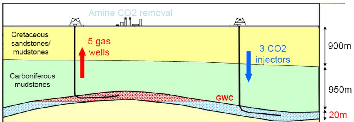
Fig.4 : Well CO<sub>2</sub> injectors at Krechba
