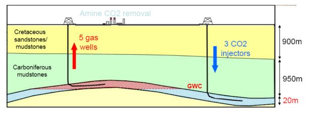
Fig.4 : Well CO2 injectors at Krechba
