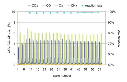
Fig. 7 The evaluation of the OC durability by continuous redox test (63 times).
