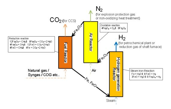
Fig. 8 New combustion system using Chemical Looping System for heat,  $N_2$  and  $H_2$  production.
