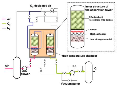
Fig. 11 The schematic diagram of HT-PSA which has heat recovery system.
