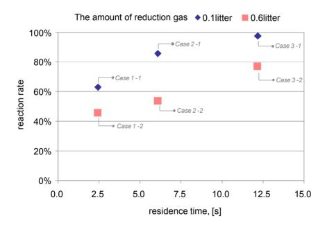
Fig. 6 The comparison of the reduction reaction rate with each residence time.
