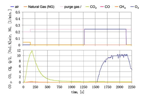
Fig. 5 The injection gas volume flow and the concentration of each gas in the exhaust gas in experimental case 3-1.
