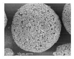
Fig. 4 SEM image of  $Fe_2O_3$  supported by  $Al_2O_3$
