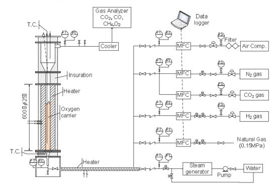
Fig. 3 The schematic diagram of chemical looping combustion test equipment
