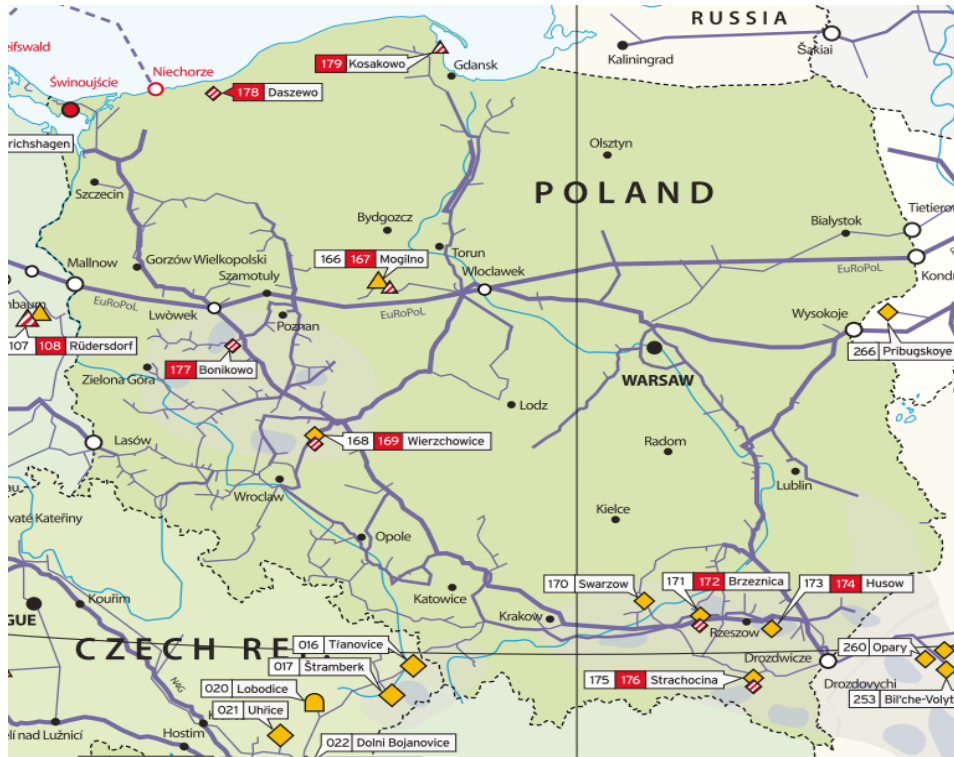
Fig. 5. Location of UGS in Poland on the background of the gas transmission system (source: Gas Infrastructure Europe)
