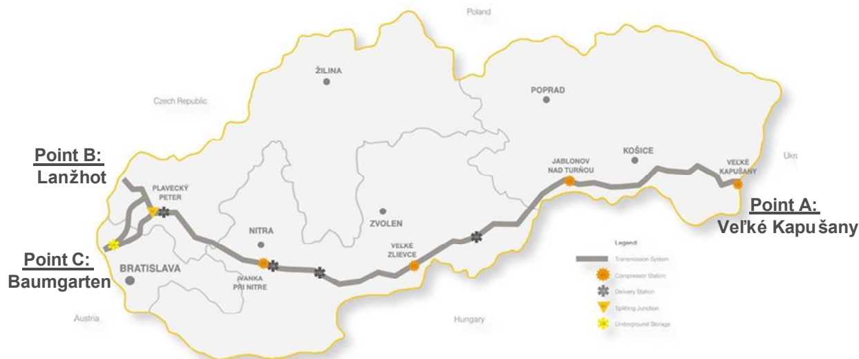
Fig. No.2. Existing Entry/Exit points of the Slovak transmission system
