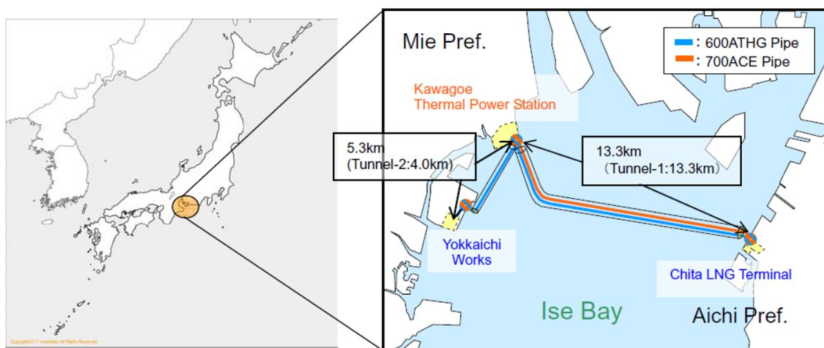
Figure 1 Schematic diagram of the route of Cross Ise Bay Gas Transmission Pipeline and existing LNG Terminal/ Thermal Power Station
