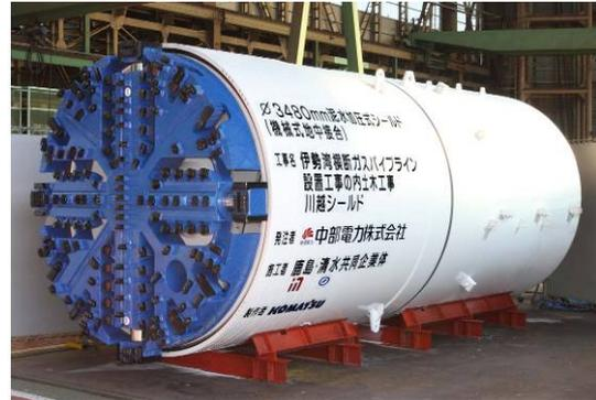
Figure 5 Structural Drawing of Machine for Kawagoe Picture 1 Shield Machine for Kawagoe
