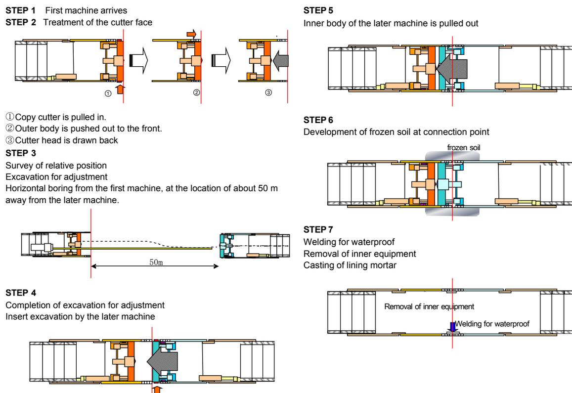
Figure 6 Construction process of Underground Docking
