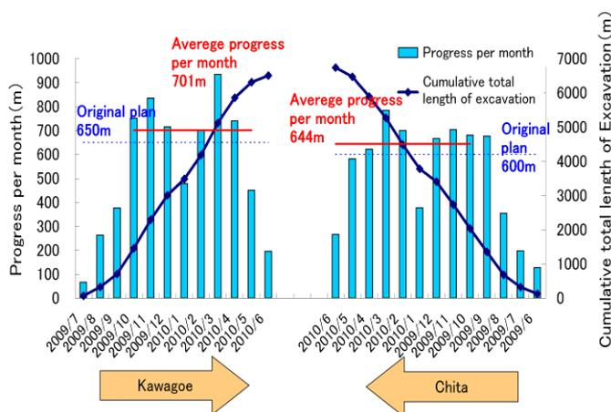
Figure 7 Record of Excavation
