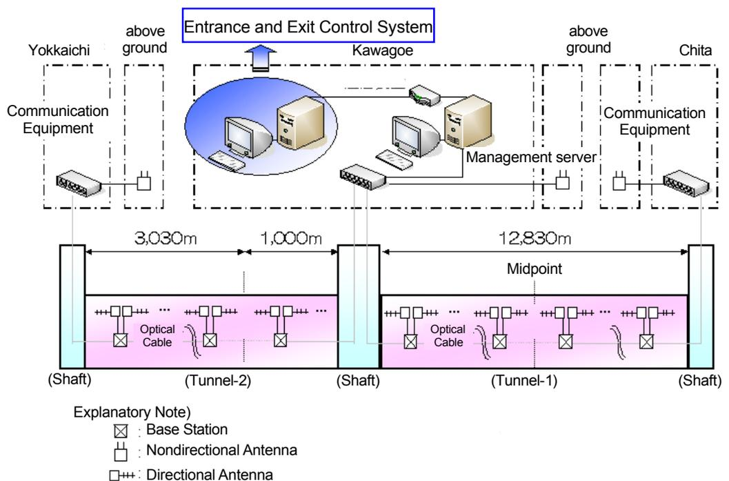
Figure 10-1 System Configuration of the Site Management System
