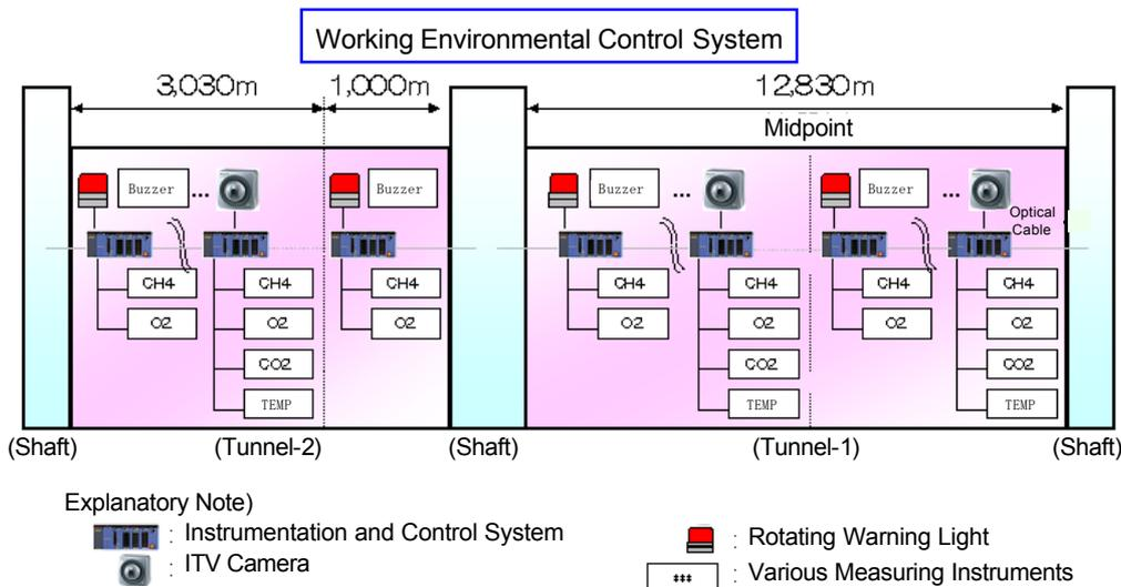
Figure 10-2 System Configuration of the Site Management System
