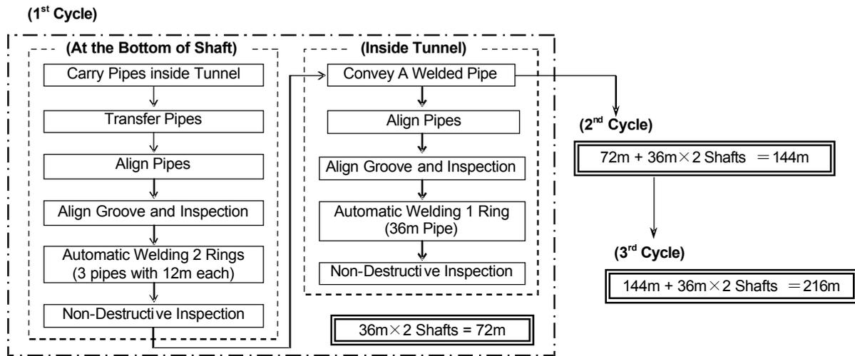
Figure 9 Workflow of Pipeline Installation inside Tunnel and Throughput
