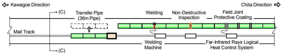
Plan View of Inside Tunnel-1 (Point (B) in the figure above )
