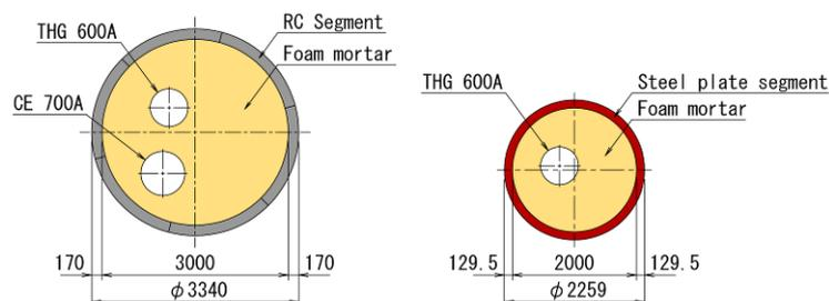
Figure 2 Cross section view of the pipeline
