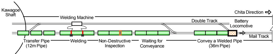
Plan View of Tunnel-1 at Bottom of Kawagoe Shaft (Point (A) in the figure above )
