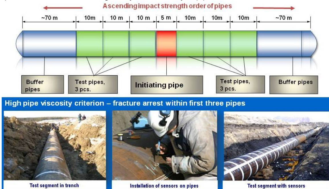
Fig.6 - Field pneumatic tests of X80 pipes
