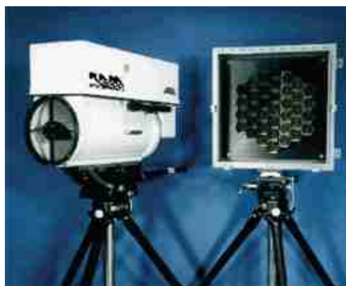
Figure 7 - Open-path FTIR source and reflector (From the EPA Clean-Up Information Technology Innovation Program website - http://clu-in.org/programs/21m2/openpath/op-ftir/ )
