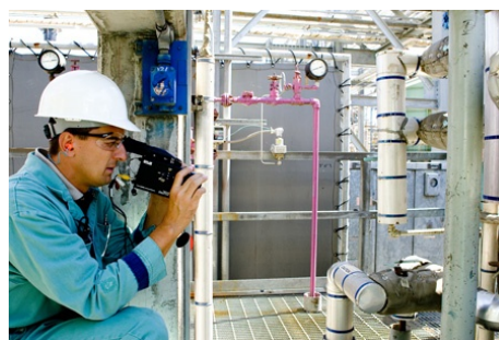
Figures 6 – Top left and right, FLIR camera depicts valve and tank leak as black smoke on the display. Bottom, technician uses a FLIR Systems, Inc. GasfindIR® (GasfindIR® registered trade mark of FLIR Systems Inc.) to survey equipment. Photos at top left and bottom courtesy of FLIR Systems, Inc. Photo at top right is from an EPA and FLIR Systems presentation 7
