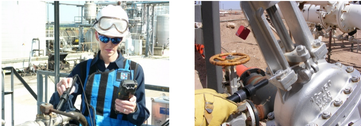
Figure 3 – Method 21 uses an organic vapor analyzer (OVA) or toxic vapor analyzer (TVA). The component is approached and, “sniffed,” to record the leak concentration. Left, a technician uses TVA to check emissions on a valve’s gasket joint. (Courtesy of Team Industrial Services, Inc.). Right, emissions from a valve’s stem seal are measured. (Courtesy of Sage Environmental Consulting.)
