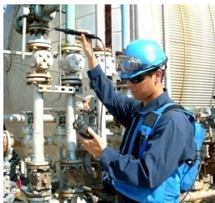
Figure 1 – Toxic vapor analyzer in use. Courtesy of Team Industrial Services, Inc.
