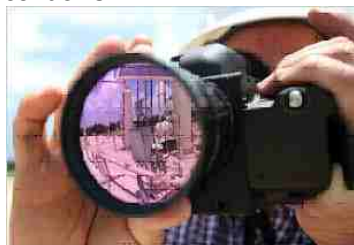
Figure 4 – Gas detecting IR camera. Courtesy of Sage Environmental Consulting.
