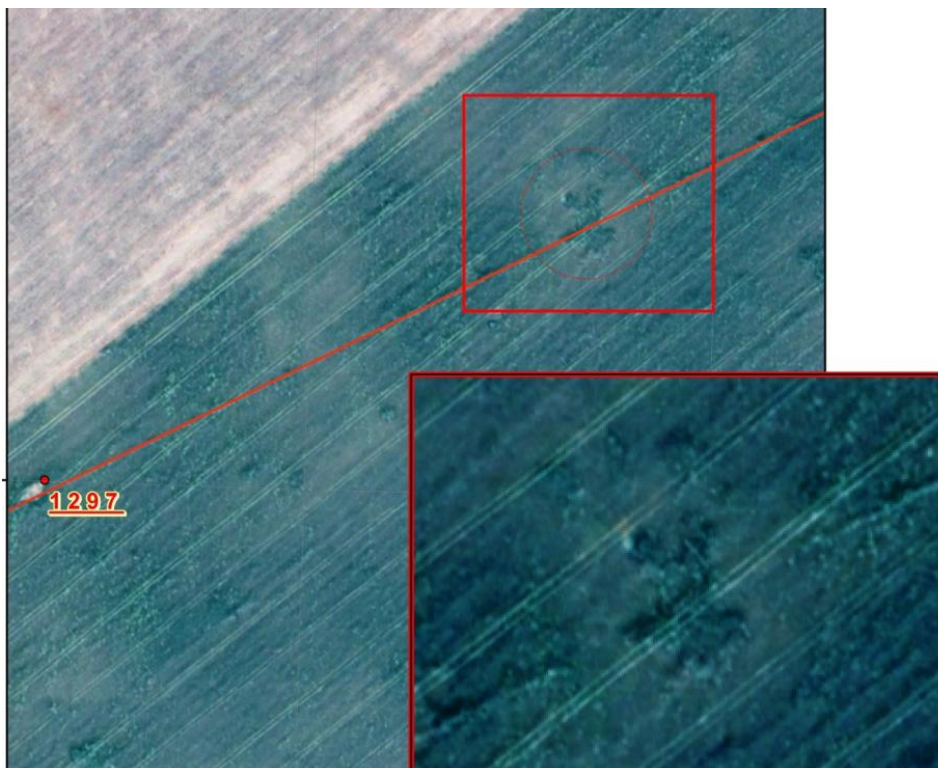
Figure 34: Circular structure on the pipeline with a high vegetation mass in its center and sharp drop in vegetation at its edges
