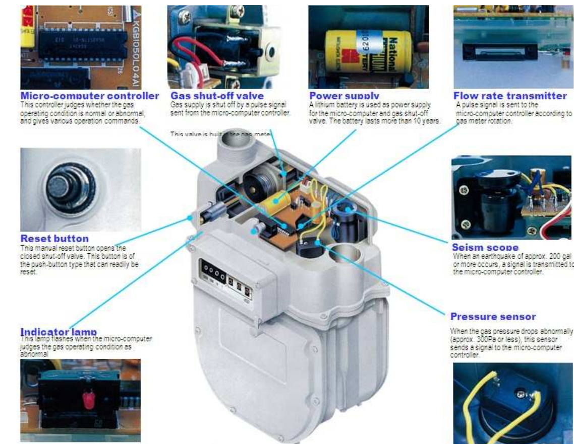
Figure 2: Structure of diaphragm type micom meter
