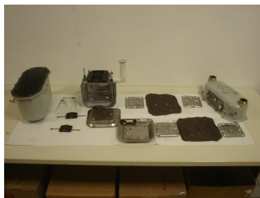
Figure 4 – Gas meter completely disassembled for the visual check
