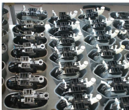
Figure 3 – Meters disassembled waiting for dimensional check and internal leak test
