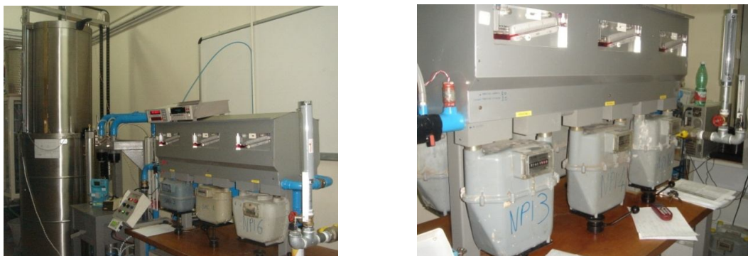
Fig.1 – Test Layout for the error of indication and pressure absorption tests
