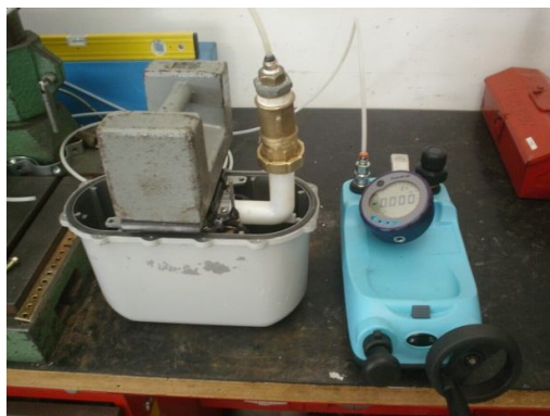
Figure 5 – Test layout for the internal pressure test
