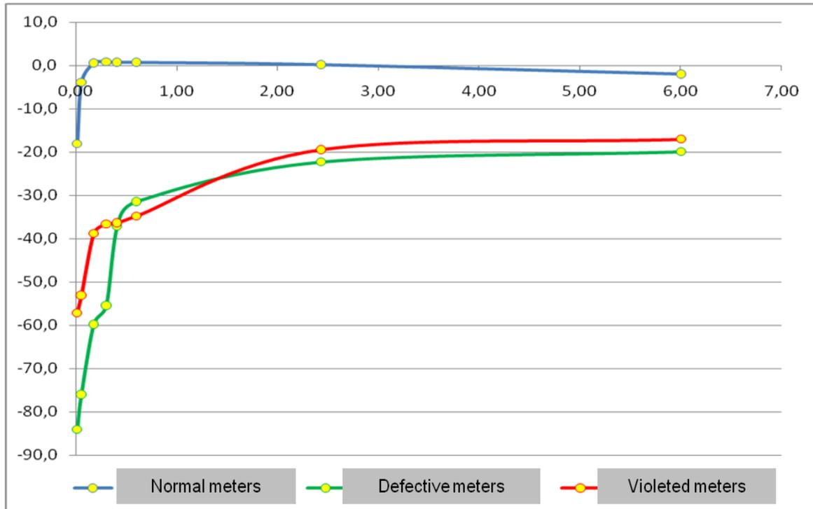
The mean values of the calibration curves according to the classification of the meter are shown in the figure below.
